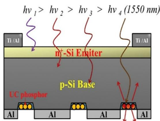
Fig. 20 A schematic diagram showing a silicon solar cell with  $\text{SiO}_2$  coating containing  $\text{YF}_3:\text{Yb}^{3+}/\text{Er}^{3+}$  phosphor particles within the backside matrix grooves for use in the upconversion of photons under excitation by a light source with a wavelength of 1550 nm. Reprinted with permission from Elsevier.<sup>77</sup>
