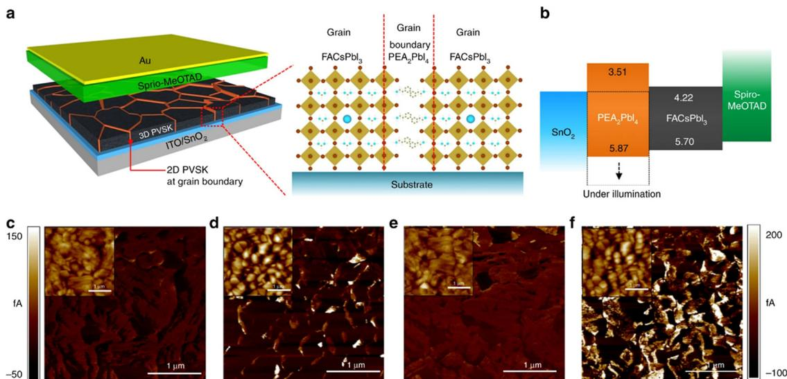
Fig. 8 Schematics of the device incorporating polycrystalline 3D perovskite film with 2D perovskite at grain boundaries and band structure of each layer in device. Reproduced from ref. 131 with permission from Springer nature, copyright 2018.
