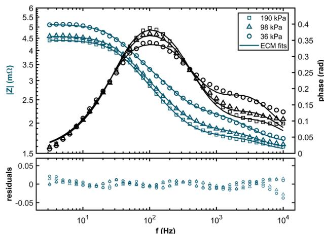
**Fig. 5** Bode plot of the impedance spectra for hydrogen partial pressures of 36 kPa, 98 kPa, and 190 kPa. The experimental data points (markers) were recorded in a frequency range between 3 Hz and 10 kHz at a current density of 1.0 A cm<sup>-2</sup>. The corresponding fits are displayed as solid curves. The corresponding relative residuals of the fits are displayed below.
