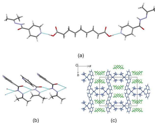
**Fig. 5** The crystal structure of izact + C9 showing (a) the hydrogen bonding between neighbouring izact molecules, (b) the hydrogen bonding between izact and C9 and (c) the packing (with izact in blue and C9 in green).
