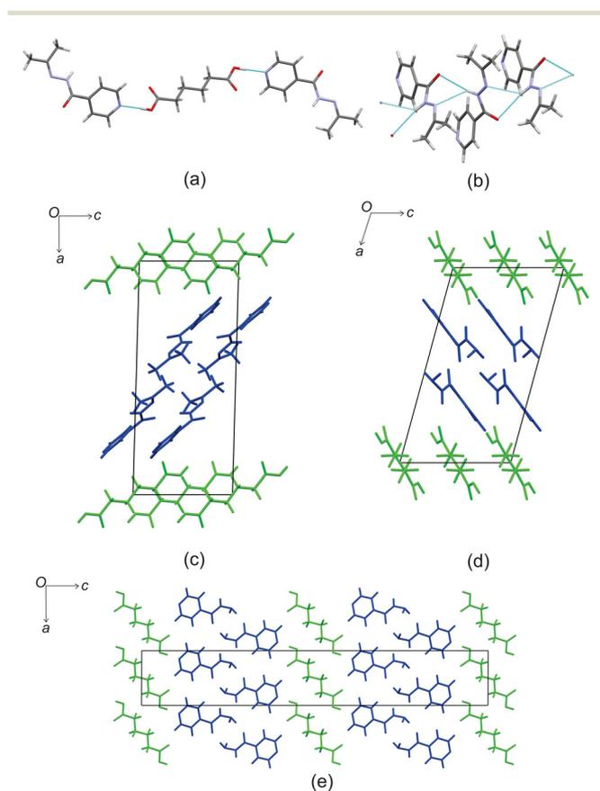
**Fig. 2** The crystal structure of izact + C6 showing (a) the hydrogen bonding between izact and C6 (b) the hydrogen bonding between neighbouring izact molecules, (c) the packing of izact + C6 (with izact in blue and C6 in green), (d) the packing of inh + C6 form II (with inh in blue and C6 in green, Refcode FADGUO01) and (e) the packing of inh + C6 form I (with inh in blue and C6 in green, Refcode FADGUO).
