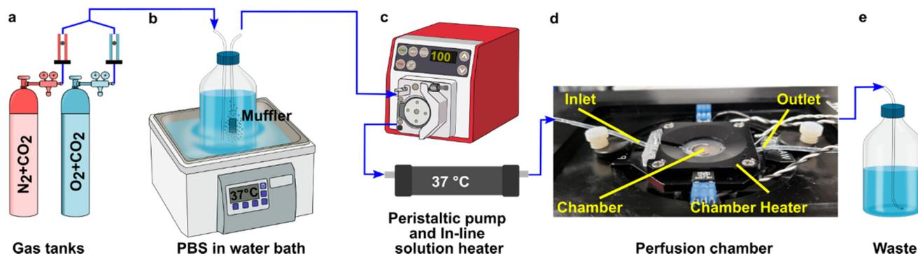
**Fig. 1** Experimental setup for imaging of oxygen consumption in tissue slices. (a) A controlled gas mixture was bubbled into (b) a PBS reservoir at 37 °C. (c) Oxygenated PBS solution was pumped into the closed imaging chamber using a peristaltic pump and is passed through an in-line heater (d) into the closed perfusion chamber with the sampler inside the chamber heater. (e) The excess PBS is collected in a waste jar.
