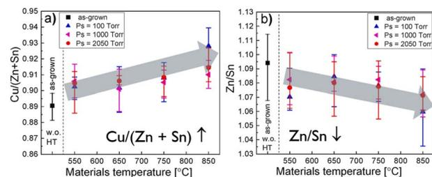
Fig. 4 (a)  $\text{Cu}/(\text{Zn} + \text{Sn})$  and (b)  $\text{Zn}/\text{Sn}$  compositional ratios of the CZTS MGP crystals depending on the post-annealing regime as determined by EDX. Reproduced from ref. 34 with permission from Elsevier B.V., Copyright 2022.
