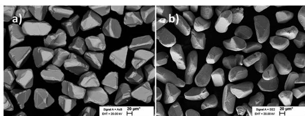
Fig. 6 SEM images of  $(\text{Cu}_{1-x}\text{Ag}_x)_{1.85}(\text{Zn}_{0.8}\text{Cd}_{0.2})_{1.1}\text{SnS}_4$  monograin powder crystals: (a)  $x = 0$  and (b)  $x = 0.15$ . Reproduced from ref. 28 with permission from the Royal Society of Chemistry, Copyright 2019.
