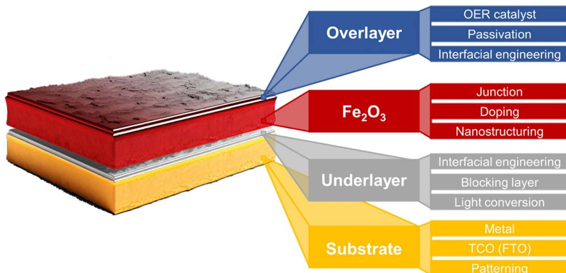
Fig. 3 Schematic illustration of various strategies for enhancing PEC efficiencies of a hematite photoanode.<sup>35–43</sup>
