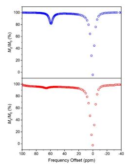
Fig. 6 CEST spectra recorded at 9.4 T of 10 mM  $\bf 1$  (top) and 30 mM  $\bf 2$  (bottom) in 50 mM HEPES buffer solution at pH 7.40 and 37 °C, with a 4 s presaturation pulse of 24  $\mu$ T.
