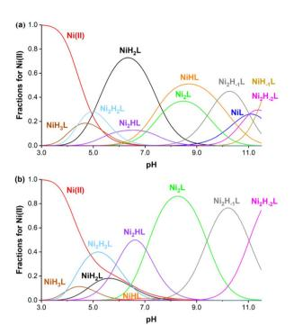
Fig. 3 Species distribution curves calculated for the Ni( $\shortparallel$ ) system at 1:1 (a) and 2:1 (b) metal-to-ligand ratios ([Ni( $\shortparallel$ )] = [Lig] = 0.002 M (upper) and [Ni( $\shortparallel$ )] = 2[Lig] = 0.002 M (bottom), 0.15 M NaCl, 25 °C). NiL and NiH<sub>-1</sub>L are not shown in (b) due to their low concentrations.
