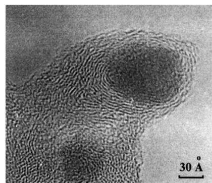
Fig. 7 TEM image of a Pd NP encapsulated in the carbon support by the “shrinkage-following-swelling” mechanism. This NP was formed via spontaneous reduction of aqueous H<sub>2</sub>[PdCl<sub>4</sub>] by the surface of the furnace NGC at 20 °C. Reproduced from ref. 32 with permission of CRC Press and Taylor & Francis Group, copyright 2003.
