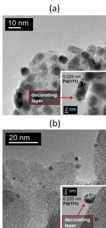
Fig. 6 TEM images at different magnifications of the 1% Pd/NGC catalysts prepared by impregnation of the carbon support with solutions of Pd<sub>3</sub>(OAc)<sub>6</sub> (a) and Pd<sub>2</sub>(dba)<sub>3</sub> (b) in chloroform followed by treatment in flowing hydrogen at 300 °C. In both cases, the Pd NPs are encapsulated by amorphous carbon formed during the high-temperature decomposition of these palladium complexes. Reproduced from ref. 47 with permission of Elsevier, copyright 2020.
