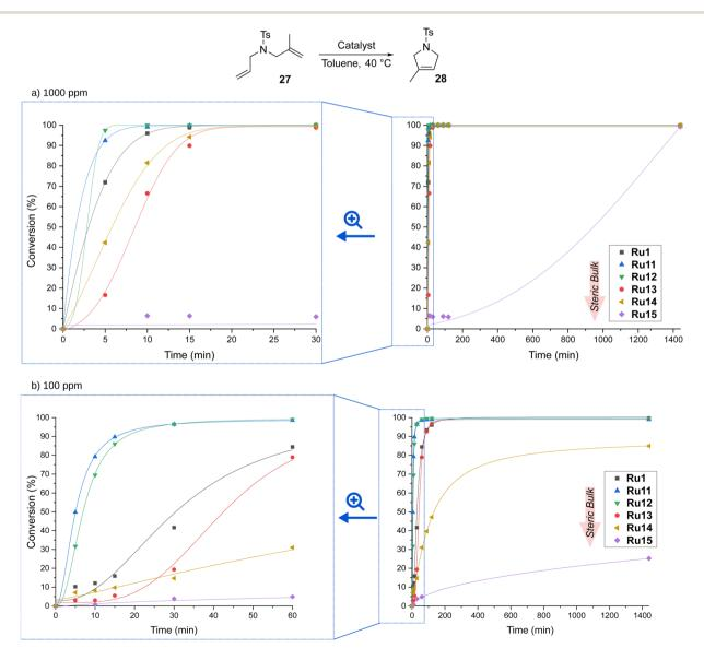
Scheme 7 Time/conversion curves for the RCM reaction of 2-allyl-2-(methylallyl)tosylate (27, 96% pure) with (a) 1000 and (b) 100 ppm of CAAC-based complexes (monitored by GC). Lines are visual aids only.
