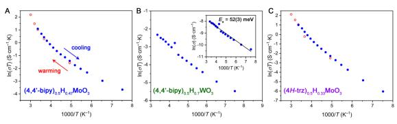
Fig. 6 Variable-temperature four-point conductivity measurements on pressed powder pellets of hybrid bronzes, plotted as  $\ln(\sigma T)$  vs. 1000/T according to the polaronic model of charge transport. (A) (4,4'-bipy) $_{0.5}H_{0.47}MoO_3$ . (B) (4,4'-bipy) $_{0.5}H_{0.7}WO_3$ . Inset: variable temperature conductivity plotted according to the linearized Arrhenius model with a fitted activation energy of conduction of 52(3) meV. (C) (4H-trz) $_{0.5}H_{0.33}MoO_3$ .
