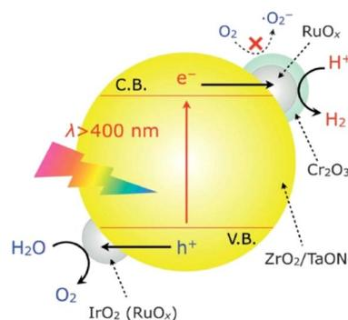
Fig. 7 Schematic of the OWS mechanism on IrO<sub>2</sub>/Cr<sub>2</sub>O<sub>3</sub>/RuO<sub>x</sub>/ZrO<sub>2</sub>/TaON. Adapted with permission from ref. 55. Copyright 2013 Wiley-VCH.
