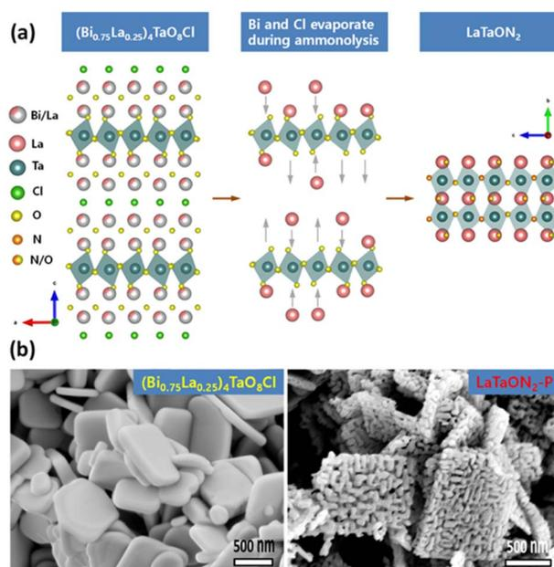
Fig. 2 (a) Schematic of structural transformation from (Bi<sub>0.75</sub>La<sub>0.25</sub>)<sub>4</sub>TaO<sub>8</sub>Cl into LaTaO<sub>2</sub>N. (b) Field-emission scanning electron microscopy images of (Bi<sub>0.75</sub>La<sub>0.25</sub>)<sub>4</sub>TaO<sub>8</sub>Cl and LaTaO<sub>2</sub>N-P. Adapted with permission from ref. 21. Copyright 2021 American Chemical Society.
