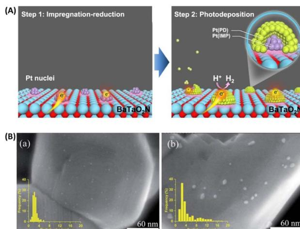
Fig. 4 (A) Schematic of sequential Pt cocatalyst deposition onto  $\text{BaTaO}_2\text{N}$ . Adapted with permission from ref. 40. Copyright 2021 Springer Nature. (B) Scanning transmission electron microscopy images and particle size distributions of (a) Na-containing and (b) Na-free Pt/ $\text{BaTaO}_2\text{N}$ . Adapted with permission from ref. 41. Copyright 2021 The Royal Society of Chemistry.
