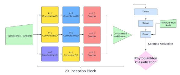
Fig. 4 The structure of neural network designed to classify phytoplankton using fluorescence transients and radii. k, w and r are kernel size, window width and dropout rate for convolution, max pooling and dropout layers, respectively.
