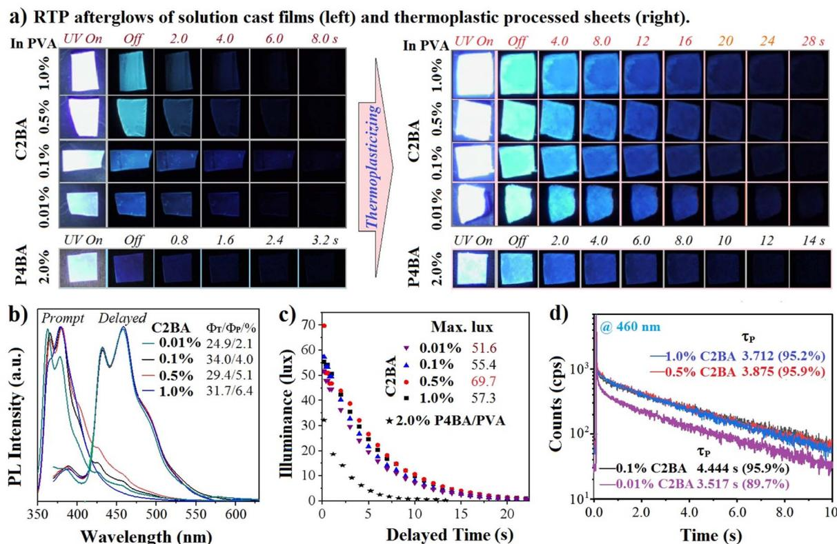
Fig. 2 (a) PL photographs of solution-cast C2BA and P4BA-doped PVA films and the corresponding thermoplastic-processed sheets with different percentages for doping weights before and after removal of 365 nm excitation light ( $0.3 \text{ mW cm}^{-2}$ ) for 5 s at room temperature in the dark. (b–d) Steady-state PL spectra, relative afterglow illuminance, time-resolved RTP decay curves, and the fitted RTP lifetimes of C2BA/PVA sheets under light excitation at 365 nm.
