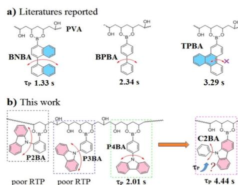
Fig. 1 (a) Structures and RTP lifetimes of arylboronic acids grafted on PVA side-chains. (b) Changing the positions of boronic acid on *N*-phenylcarbazole to suppress the internal rotation of a triplet chromophore and boost the RTP lifetime to a higher level.
