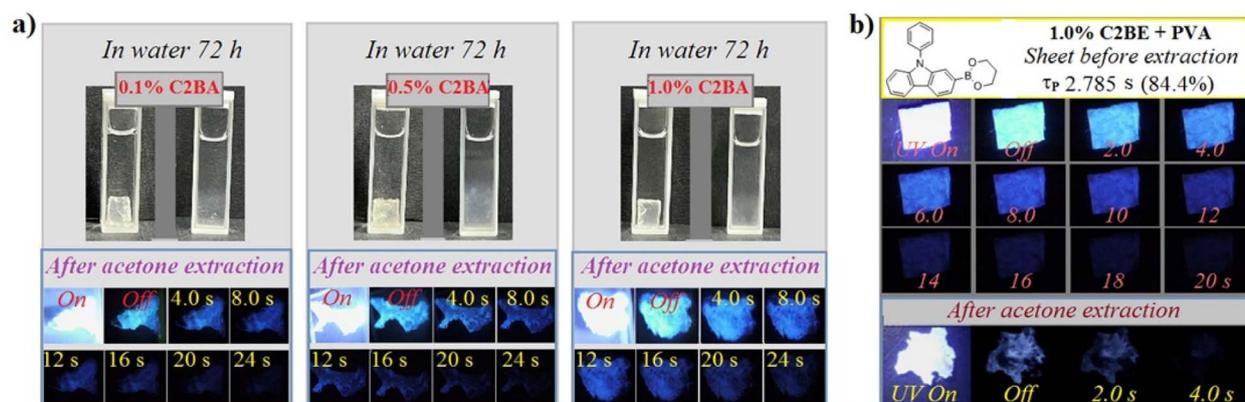
Fig. 3 (a) Dissolution photographs of C2BA/PVA sheets in water and the corresponding residue PL photographs after acetone extraction. (b) PL photographs of a C2BE/PVA sheet and its residue after dissolution-extraction. Samples were excited by light at 365 nm at room temperature.
