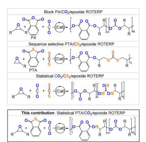
Fig. 1 Comparison of the literature-reported ROTERP and the ROTERP presented in this contribution; [Li] = LiOCH<sub>2</sub>Ph (LiOBn), R = Me, Et,  $-(C_aH_B)-$ .
