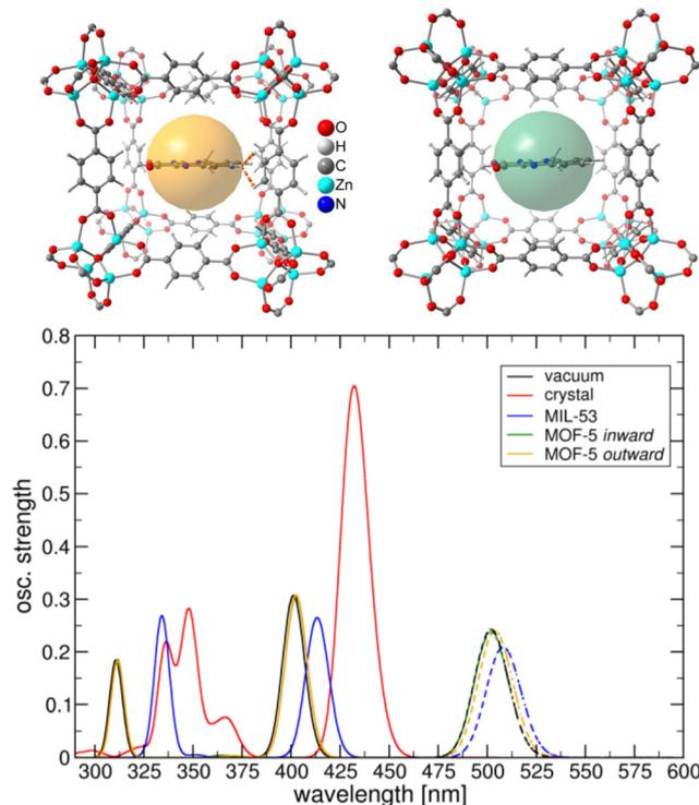
**Fig. 16** DFT/MRCI absorption spectra (BHLYP/TZVP) using the R2016 Hamiltonian of MIA fluorophore in vacuum, crystal, and MOF (MIL-53 and MOF-5) environments. The clusters were obtained using a hybrid QM/MM (PBE0/AMBER16) geometry optimisation, where the *model* region was the fluorophore dye. The phenyl linkers in MOF-5 in the MOF can point in the inward (left) and outward cage configurations. Modified from ref. 122, with permission.
