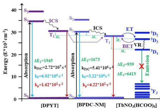
Fig. 15 Energy level diagram of the most likely sensitisation and emission pathway obtained by Hildago-Rosa *et al.* using a multireference CAS(8,7)SCF/NEVP2 and TD-B3LYP/def2-TZVPP/CPCM protocol. Reprinted with permission from ref. 3. Copyright 2022 American Chemical Society.
