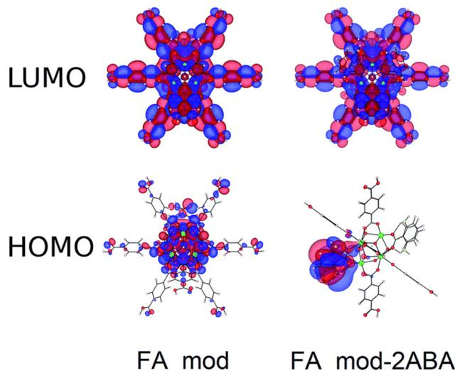
Fig. 20 Defect functionalisation of UiO-66 introduces a new HOMO localised on the site of the aminobenzene defect, improving selectivity in photocatalytic CO<sub>2</sub>-to-CO conversion. Visualisations obtained using TD-PBE/DZP-MOLPLOT-SR-GTH/GTH-PBE cluster calculations using the GPW method. Reproduced from ref. 235 with permission from Royal Society of Chemistry, copyright 2019.
