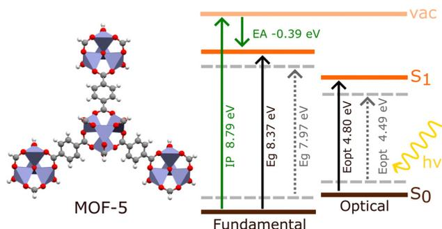
Fig. 3 Schematic comparing the optical ( $E_{\text{opt}}$ ) and fundamental ( $E_{\text{g}}$ ) band gaps obtained from BSE/evGW/PBE0 h-capped cluster model (bold lines) and BSE/evGW/Gau-PBE periodic model (dashed lines) calculations in MOF-5, obtained by Kshirsagar *et al.* (ref. 74). The ionisation potential (IP) and electron affinity (EA) obtained for the cluster model are also shown. The periodic IP of MOF-5 has been previously reported as 7.30 eV (HSE06).<sup>75</sup>
