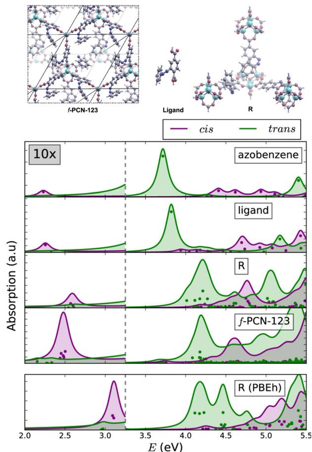
Fig. 5 Comparison of the BSE/evGW/PBE spectra of azobenzene, a single ligand, a cluster of SBUs, and a fully periodic model. The lowest panel was performed at the BSE/evGW/PBEh level (including 40% HF exchange). These results show the capacity of cluster models to recover key features of the optical absorption spectrum of the fully periodic wavefunction. Adapted with permission from ref. 109. Copyright 2020 American Chemical Society.
