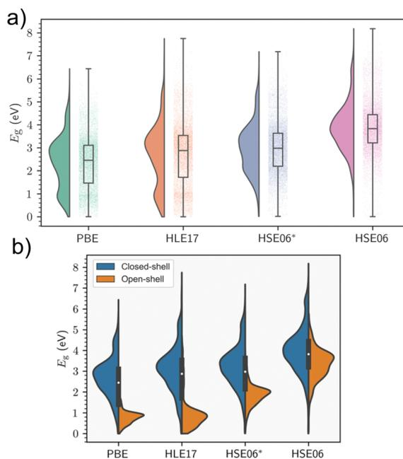
Fig. 13 (a) Distribution of band gaps,  $E_g$ , for the 10720 structures found within the QMOF database, determined using periodic DFT using GGA (PBE), meta-GGA (HLE17), and hybrid (HSE06, HSE06\*) functionals, and (b) decomposed into the closed- and open-shell contributions. Adapted with permission figure from ref. 83. IOP Publishing. Reproduced with permission. All rights reserved.
