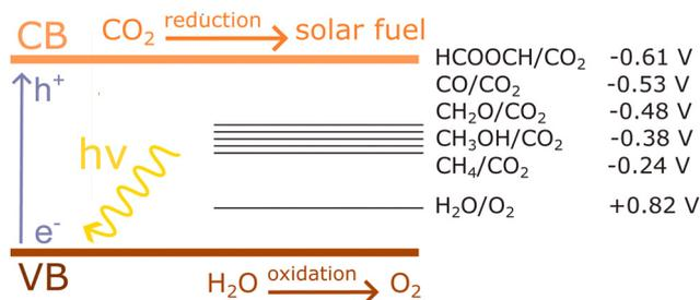
Fig. 18 The general scheme for the photochemical carbon dioxide reduction reaction (CO<sub>2</sub>RR). The reduction potentials are from ref. 216.
