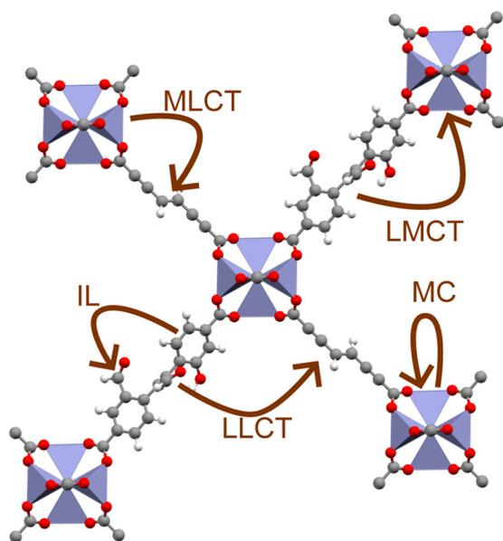
**Fig. 1** Different types of charge transfer available in MOFs: ligand-to-metal charge transfer (LMCT); metal-to-ligand charge transfer (MLCT); ligand-to-ligand charge transfer (LLCT); intra-ligand charge transfer (IL); and metal-centred charge transfer (MC).
