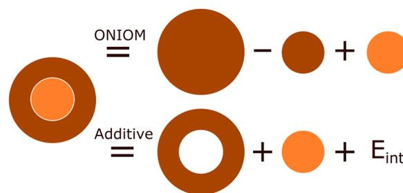
Fig. 9 Two-layer hybrid model methods extrapolate a high-level of theory (orange) of a *model* region to the complete *real* system, which is simulated at a low-level of theory (brown). The ONIOM scheme accounts for interactions between these subsystems implicitly *via* subtraction in the total Hamiltonian, whereas the additive scheme treats the *model* and *env* systems separately, with an explicit energetic coupling term,  $E_{\text{int}}$ .
