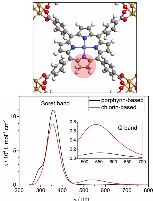
Fig. 19 Simulated TD-HSE06/6-311G(d,p) spectra for porphyrin- and chlorin-based M-TCPP. Chlorin has a similar structure to porphyrin, however one pyrrole group hydrogenated (highlighted in red) in chlorin. Modified figure from ref. 90.
