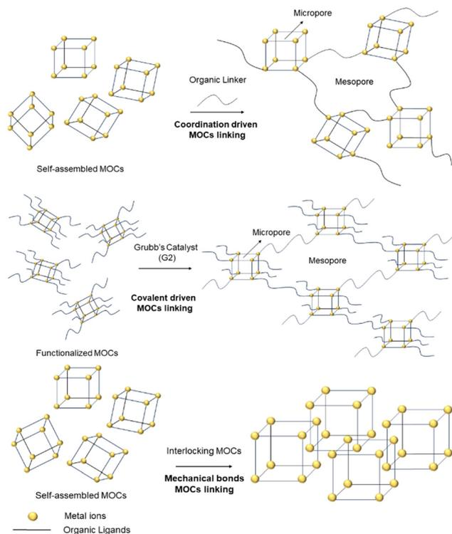
Fig. 1 Cartoon showing the stepwise synthesis of connected **MOCs** *via* ligand coordination (top), covalent bond formation from functionalized **MOCs** (middle) and interlocking of **MOCs** *via* mechanical bonds (bottom).
