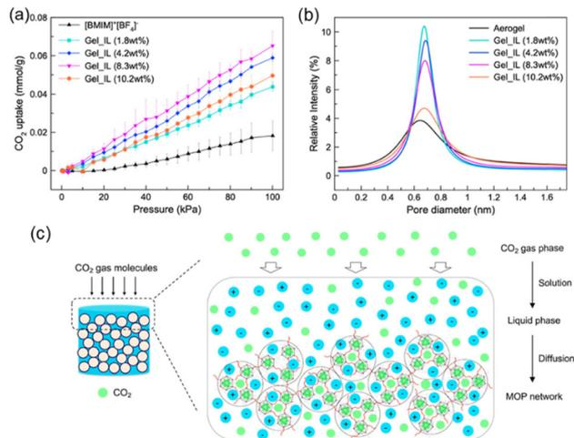
Fig. 5 (a) CO<sub>2</sub> uptake isotherms of Gel\_IL at different concentrations of **MOC-2** networks at 303 K under 100 kPa. (b) Particle size distribution of Gel\_IL with different concentrations of **MOC-2** networks derived from PALS experiments. (c) Cartoon representing the CO<sub>2</sub> gas diffusion pathway within the wet sample of connected **MOCs**. Reproduced from ref. 51 with permission from ACS, copyright 2023.
