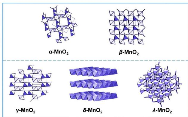
Fig. 4 Crystal structures of  $\alpha\text{-MnO}_2$ ,  $\beta\text{-MnO}_2$ ,  $\gamma\text{-MnO}_2$ ,  $\delta\text{-MnO}_2$ , and  $\lambda\text{-MnO}_2$ . Reprinted with permission from ref. 110. Copyright 2018, Elsevier.
