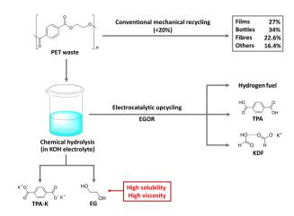
Fig. 5 Electrocatalytic PET upcycling to commodity chemicals and  $\rm H_2$  fuel. Reproduced with permission from ref. 51. Copyright 2021 Springer Nature.
