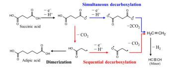
Fig. 10 Anodic decarboxylation pathways of succinic acid produced by the depolymerization of PE. Reproduced with permission form ref. 27. Copyright 2021 ACS publications.
