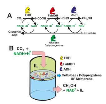
Fig. 6 (A) Scheme of a multi-enzyme system for methanol synthesis from  $CO_2$  with *in situ* regeneration of NADH. (B) Set-up of the proposed IL-based multi-enzymatic membrane reactor for  $CO_2$  transformation to methanol.<sup>80</sup>
