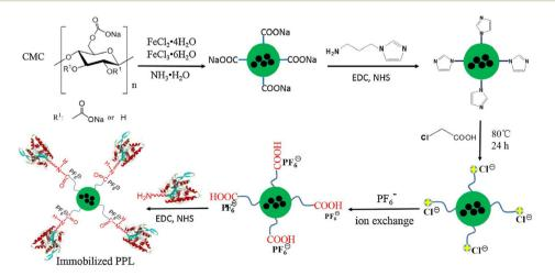
Fig. 12 Enzyme (porcine pancreatic lipase (PPL)) immobilisation on carboxymethylcellulose-coated magnetic nanoparticles via an ionic liquidderived anchor. Reproduced with some modification from ref. 129 with permission from Elsevier, copyright 2020.
