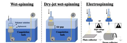
Fig. 29 Common spinning techniques for fabricating synthetic cellulose fibres from solutions. Other methods, such as dry-jet spinning uses no coaqulation bath, and for melt spinning the polymer melt is extruded through the spinneret (note that this is not possible for cellulose itself).
