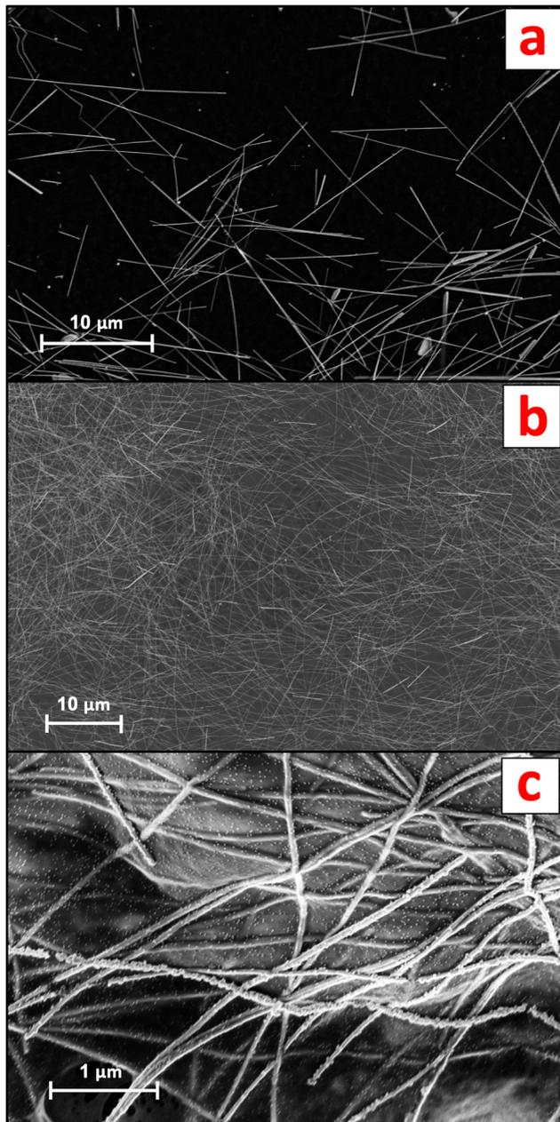
**Fig. 1** Scanning electron microscopy analysis of the pristine ENMs and NEPs in this study. (a) The pristine AgNW standard (7 kV, VP BSE detector). (b) The homogeneous surface distribution of AgNWs onto the AgNWs-PPE cellulose matrix (7 kV, VP BSE detector). (c) A close-up of the AgNWs at the AgNWs-PPE surface (0.5 kV, in-lens SE detector).
