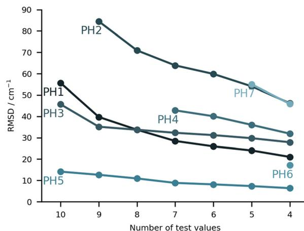
**Fig. 5** RMSD values (in  $\text{cm}^{-1}$ ) for the purely harmonic (PH) submissions. The values are provided incrementally removing the worst prediction of each set, in order to compare in a more balanced way the different submissions.
