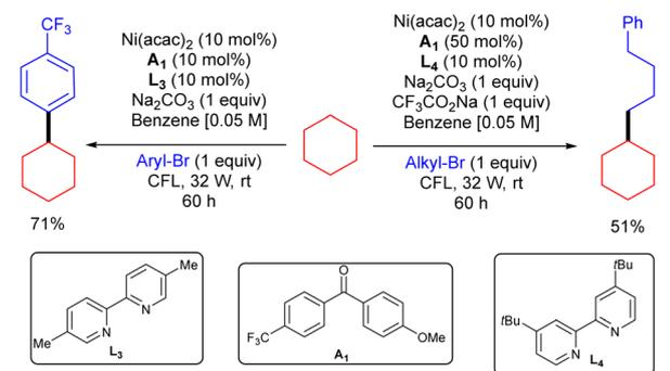
**Scheme 39** Ni/ketone-catalysed C(sp<sup>3</sup>)-H arylation and alkylation of alkanes.
