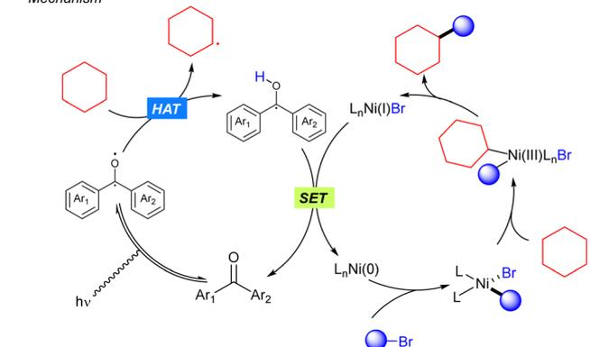
**Scheme 39** Ni/ketone-catalysed C(sp<sup>3</sup>)-H arylation and alkylation of alkanes.
