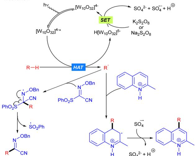
Scheme 25 Heteroarylation of alkanes based on TBADT/S<sub>2</sub>O<sub>8</sub><sup>2-</sup> catalysis.
