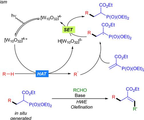
Scheme 27 Two-step photocatalytic Michel addition/HWE olefination in flow.
