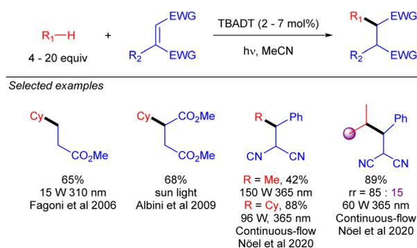
Scheme 22 TBADT-catalysed radical conjugate addition of alkanes.
