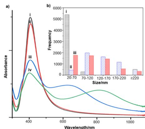
**Fig. 4** (a) UV-vis absorption spectra of Ag colloid, (i) Unaggregated (ii) with *S. aureus* *es*-biofilm, (iii) with *S. aureus* *es*-biofilm and after addition of 1 M MgSO<sub>4</sub> and (iv) after addition of 1 M MgSO<sub>4</sub> only. (b) Particle size distribution of Ag colloid (i) before aggregation, (ii) after addition of 1 M MgSO<sub>4</sub> and (iii) with *S. aureus* *es*-biofilm after addition of 1 M MgSO<sub>4</sub>.
