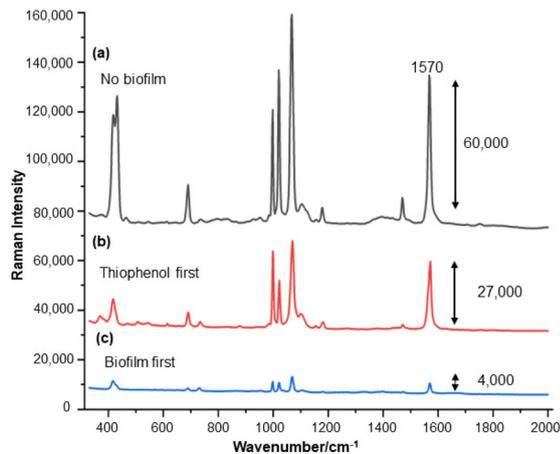
**Fig. 5** SERS spectra of  $10^{-4}$  M thiophenol on Ag colloid aggregated with 1 M  $\text{MgSO}_4$ . (a) Thiophenol only, (b) thiophenol-treated sample after addition of *S. aureus* *es*-biofilm (c) sample where *S. aureus* *es*-biofilm was added to colloid before addition of thiophenol.
