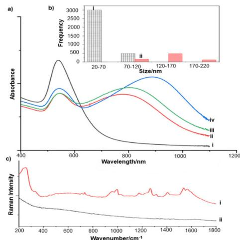
**Fig. 6** (a) UV-vis absorption spectra of Au colloid, (i) Unaggregated (ii) with *S. aureus* *es*-biofilm, (iii) with *S. aureus* *es*-biofilm and after addition of 1 M  $\text{MgSO}_4$  and (iv) after addition of 1 M  $\text{MgSO}_4$  only. (b) Particle size distribution of Au colloid (i) before aggregation, (ii) after addition of *S. aureus* *es*-biofilm. (c) SERS spectra of Au colloid (i) and Ag colloid (ii) after addition of *S. aureus* *es*-biofilm with no additional salt.
