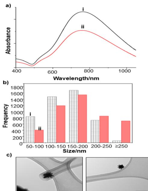
Fig. 7 (a) UV-vis absorption spectra of NS colloid, (i) Unaggregated (ii) with *S. aureus es*-biofilm (b) Particle size distribution of NS colloid (i) before aggregation, (ii) after addition of *S. aureus es*-biofilm. (c) TEM image of the NS colloid. Scale bar = 100 nm.
