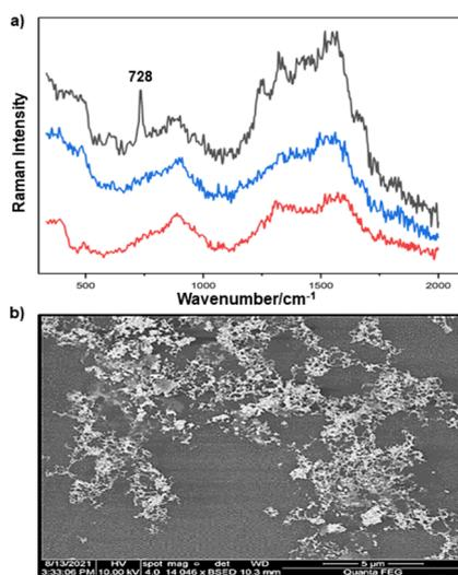
Fig. 1 (a) Au colloid-enhanced spectra recorded at three different positions of an *in situ* *S. aureus* biofilm. (b) SEM image of AuNPs adsorbed onto the surface of *S. aureus* biofilm. Scale bar =  $5\ \mu\text{m}$ .
