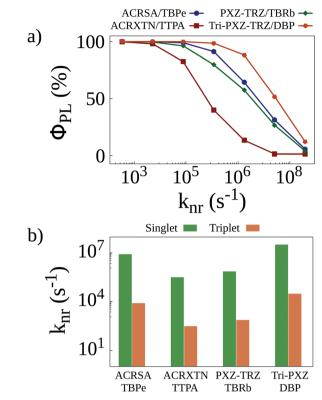
Fig. 3 (a) Photoluminescence quantum yields as a function of the non-radiative decay rate for singlet excitons calculated for simulations with initially only singlet excitons. (b) Non-radiative decay rates that better reproduce experimentally obtained quantum yields<sup>8</sup> as a function of the energy of the emission peak of the four TADF/emitter pairs.
