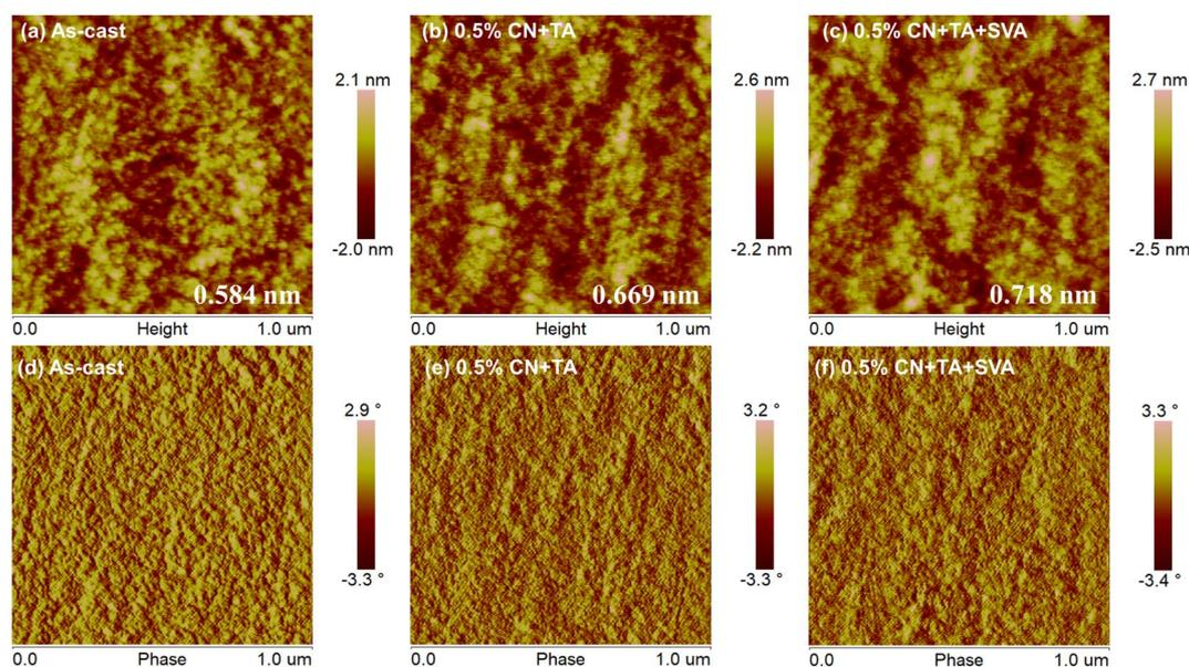
Fig. 3 (a-c) AFM height and (d-f) phase images of binary PTQ10:Y26 blend films with different treatment conditions.
