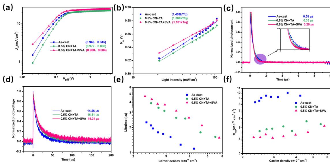
Fig. 5 (a) Photocurrent density ( $J_{ph}$ ) as a function of effective voltage ( $V_{eff}$ ) characteristics. (b) Light intensity dependence of  $V_{oc}$ . (c) Transient photocurrent and (d) transient photovoltage decay curves of the PTQ10:Y26 devices under different treatments. (e) Charge carrier lifetime versus charge density. (f) Bimolecular recombination rate constant  $k_{rec}$  versus different charge densities of PTQ10:Y26 devices.
