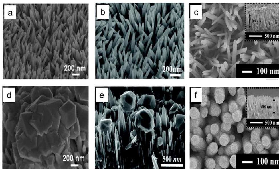
Fig. 9 (a)–(c) SEM images of ZnO nanostructures. (d)–(f) SEM images of the respective ZnTe-overcoated nanostructures (a) and (d) are reproduced with permission from Jang *et al.*,<sup>133</sup> Copyright 2014, John Wiley and Sons, (b) and (e) are from Jang *et al.*,<sup>134</sup> Copyright 2015, Royal Society of Chemistry, (c) and (f) are from Jang *et al.*,<sup>135</sup> Copyright 2016, American Chemical Society.
