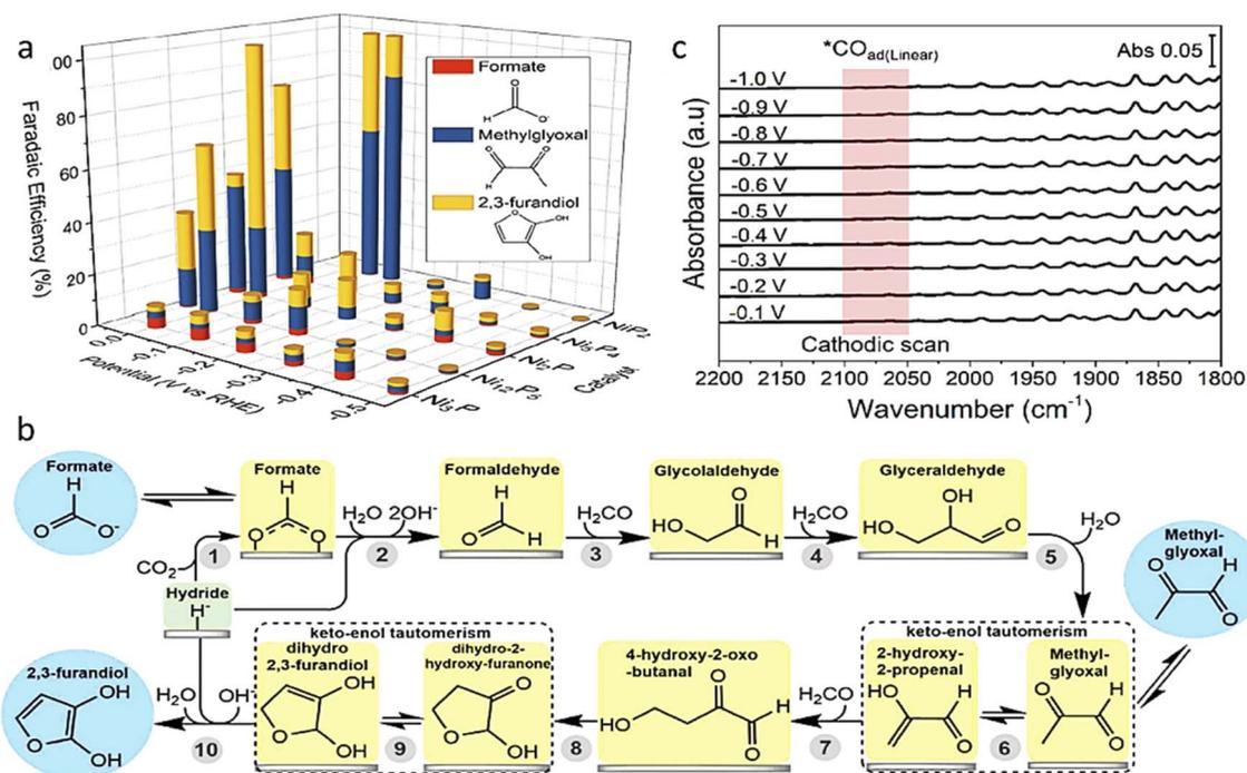
Fig. 14 (a) FEs at different potentials for different phosphide materials. (b) A predicted mechanism where products are given with blue backgrounds, and O-bound intermediates are presented with yellow backgrounds. (c) An *in situ* SEIRS study at different potentials. (a), (b) Reproduced with permission from Calvinho *et al.*,<sup>193</sup> Copyright 2018, Royal Society of Chemistry; and (c) from Choi *et al.*,<sup>194</sup> Copyright 2021, American Chemical Society.
