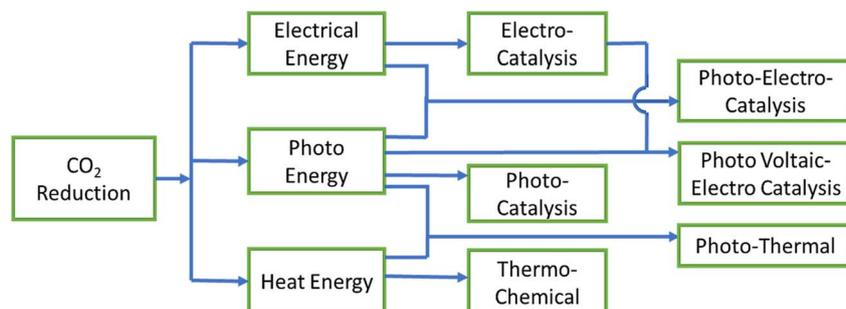
Fig. 1 The fundamental differences between CO<sub>2</sub>RR processes with respect to energy utilization.
