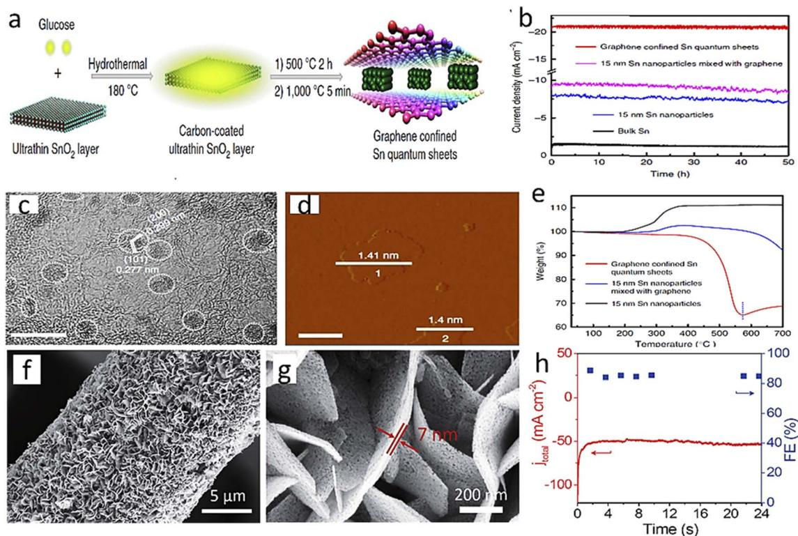
Fig. 12 (a) A schematic diagram of a synthetic procedure. (b) 50 h chronoamperometry data at  $-1.8 V_{SCE}$ . (c) A HRTEM image (10 nm scale). (d) An AFM image. (e) TGA data. (f), (g) SEM images of mesoporous  $SnO_2$  nanosheets. (h) The chronoamperometry curve over long-term testing, (a)–(e) are reproduced with permission from Lei *et al.*,<sup>181</sup> Copyright 2016, Springer Nature Limited, and (f)–(h) from Li *et al.*,<sup>183</sup> Copyright 2016, John Wiley and Sons.
