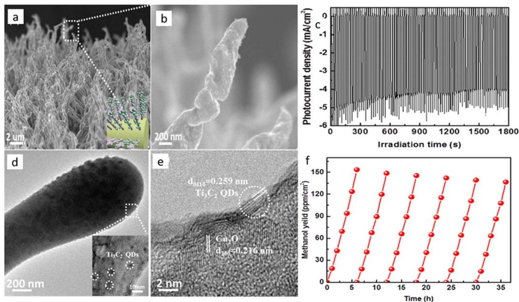
Fig. 8 (a), (b) SEM images of  $\text{Ti}_3\text{C}_2$  QD loaded  $\text{Cu}_2\text{O}$  NWs. (c) The photocurrent vs. time curve. (d), (e) TEM images of the same composite. (f) Recyclability data over 6 cycles. Reproduced with permission from Zeng *et al.*,<sup>120</sup> Copyright 2018, John Wiley and Sons.
