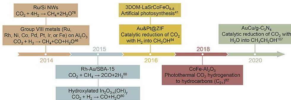
Fig. 2 A timeline of the advances in photothermal catalytic  $\text{CO}_2$  reduction. Reprinted with permission from Zhang *et al.*,<sup>51</sup> Copyright 2021, Elsevier Ltd.
