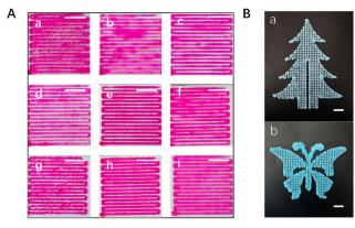
Fig. 3 Digital images of 3D-bioprinted (A) parallel strands of pre-cured hydrogels, a.b-6%-0-1h, b.b-6%-0-1.5 h, c.b-6%-0-2h, d.b-8%-0.3-1h, e.b-8%-0.5-1h, f.b-8%-0.7-1h, g.b-10%-0.8-1h, h.b-10%-1.0-1h, and i.b-10%-1.2-1h, "b" refers to "3D-bioprinted", and (B) multi-layered complex structures in a tree shape (a) and a butterfly shape (b). The scale bar is 1 cm.
