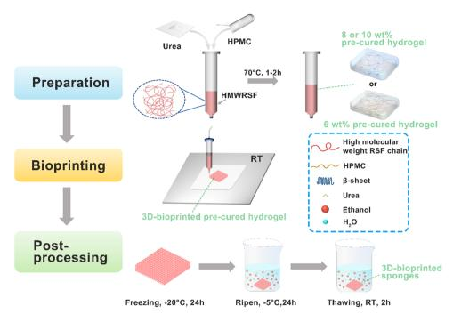
Fig. 1 Schematic illustration of the preparation, bioprinting, and post-processing procedure of HMWRSF-based pre-cured hydrogels. HMWRSF: highmolecular-weight regenerated silk fibroin, HPMC: hydroxypropyl methylcellulose, and RT: room temperature. Urea was not introduced for a 6 wt% precured hydrogel.
