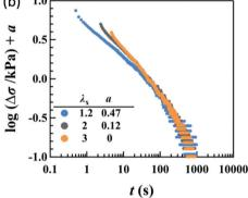
Fig. 8 (a) Total stress relaxation ( $\Delta \sigma^{\infty}$ ) in uniaxial stretching as a function of  $\lambda_{x}$ for the HG gels with  $X_{CD} = 0.63$  and various concentrations of covalent crosslinks. (b) Failure of the superposition of  $\log \Delta \sigma$  –  $\log t$  curves for uniaxial stretching with various values of  $\lambda_x$  by vertical shift with a factor of a for HGG63-2.
