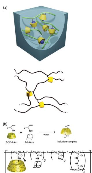
Fig. 1 Schematics of the (a) (top) HG gel with the inclusion complex and permanent rotaxane cross-link (HGG); (bottom) Gel with permanent rotaxane cross-link without the inclusion complex (CDG-0). (b) Scheme of the formation of the inclusion complex and the chemical structure of the gel specimens
