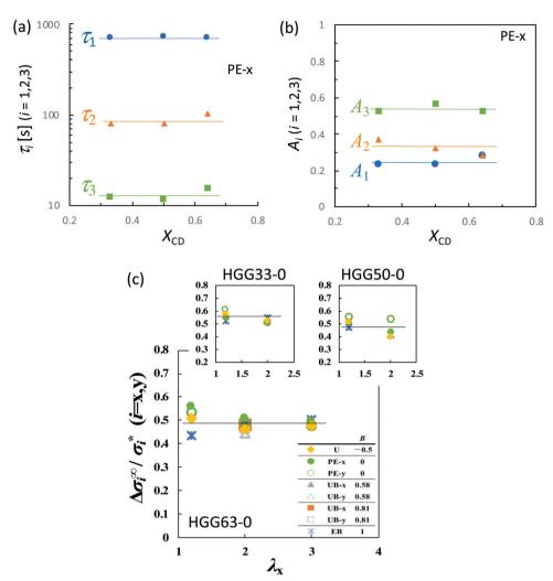
Fig. 7 (a) Relaxation times,  $\tau_i$  (i=1,2, and 3) and (b) relaxation strengths,  $A_i$  (i=1,2, and 3) as a function of  $X_{\text{CD}}$  for  $\sigma_x$  in planar extension. (c) Total stress relaxation ( $\Delta\sigma^{\infty}$ ) in several types of stretching as a function of  $\lambda_x$  for the HG gels with various values of  $X_{\text{CD}}$ .  $\Delta\sigma^{\infty}$  is reduced by the initial stress ( $\sigma^*$ ) in each deformation.
