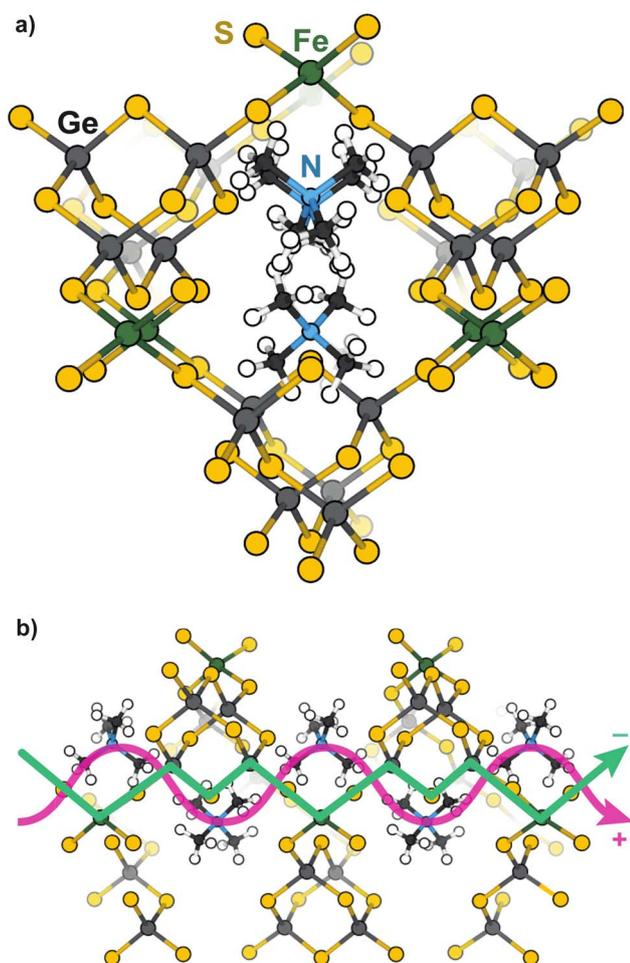
Scheme 1 Representations of  $\text{TMA}_2\text{FeGe}_4\text{S}_{10}$  viewed along the (a) [100] and (b) [101] directions. Proposed conduction pathways of delocalized electrons and extra-framework cations are highlighted in green and pink, respectively.
