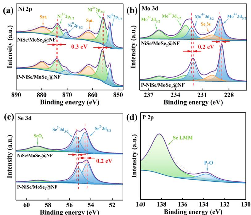
Fig. 3 XPS spectra of (a) Ni 2p, (b) Mo 3d, (c) Se 3d in NiSe/MoSe<sub>2</sub>@NF and P-NiSe/MoSe<sub>2</sub>@NF. (d) XPS spectrum of P 2p in P-NiSe/MoSe<sub>2</sub>@NF.
