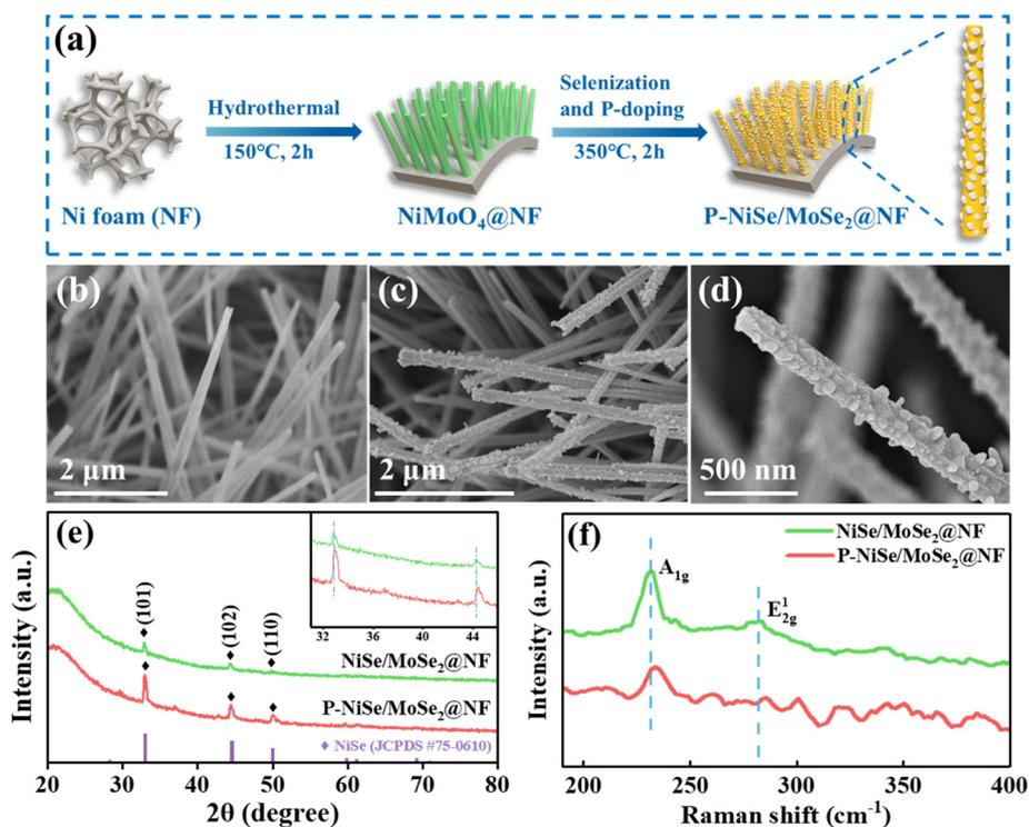
**Fig. 1** (a) Schematic of the synthesis of the P-NiSe/MoSe<sub>2</sub>@NF electrode. SEM images of (b) NiMoO<sub>4</sub>@NF and (c and d) P-NiSe/MoSe<sub>2</sub>@NF. (e) XRD patterns and (f) Raman spectra of NiSe/MoSe<sub>2</sub>@NF and P-NiSe/MoSe<sub>2</sub>@NF.
