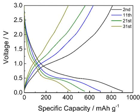
Fig. 10 GDC profiles of #3 in LP30 at 100 mA g<sup>-1</sup>.
