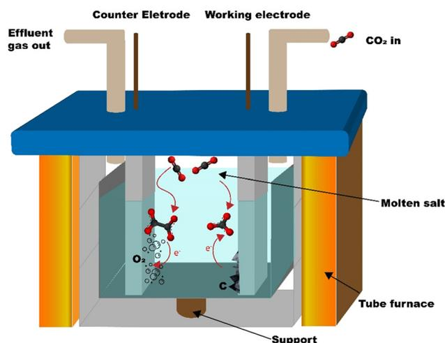
Fig. 1 Schematic of the MSCC-ET reactor.
