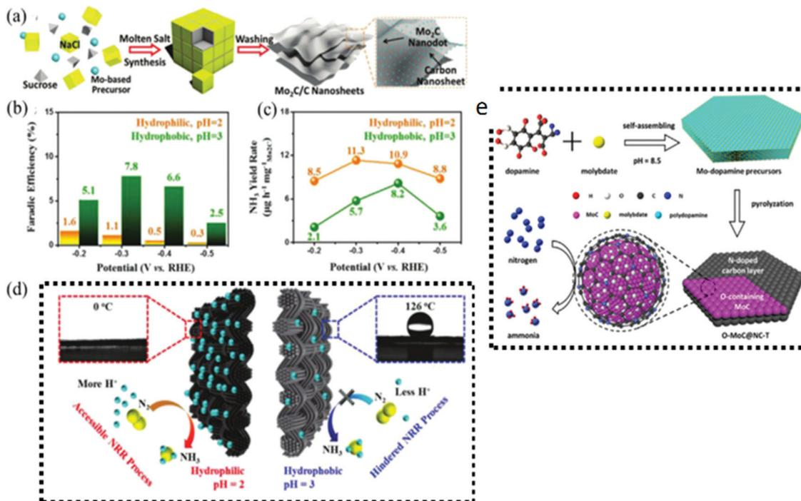
**Fig. 8** (a) Schematic representation of the synthetic route for molten salt Mo<sub>2</sub>C/C nanosheets. (b) Faradaic efficiency, (c) yield rate and (d) NRR mechanistic pathway of Mo<sub>2</sub>C/C in proton-suppressed and enriched environments. Reproduced with permission,<sup>130</sup> Copyright 2018, Wiley-VCH Verlag GmbH. (e) Schematic illustration of the fabrication procedure of OeMoC@NC-T. Reproduced with permission,<sup>135</sup> Copyright 2019, American Chemical Society.
