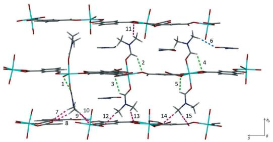
Fig. 3 Hydrogen bonding in 1. The three types found within the structure are shown in different colours: blue shows the hydrogen bond (6) between the coordinated DMF and the solvent DMF, green the intramolecular hydrogen bonds (1–5) from the coordinated DMF t to the carboxylate oxygen, and pink the hydrogen bonds (7–15) between the axially bound DMF molecules to the carboxylate oxygen atoms of subsequent layers. The numbers correspond to those given in Table S2.‡
