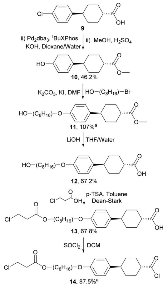
**Scheme 4** The synthesis of aligning mesogenic arm unit, <sup>a</sup>product used without purification - crude yield given.
