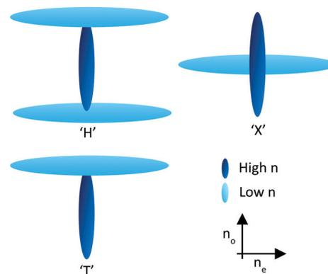
Fig. 3 Representation of H, X and T shaped materials.
