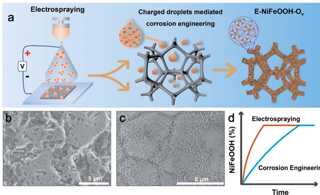
Fig. 1 (a) Schematic illustration of the reaction process of E-NiFeOOH composites *via* electrospaying. (b) SEM images of I-NiFeOOH-20 min. (c) SEM images of E-NiFeOOH-20 min. (d) The content (%) of NiFeOOH changes over time in different systems: electrospaying and corrosion engineering.
