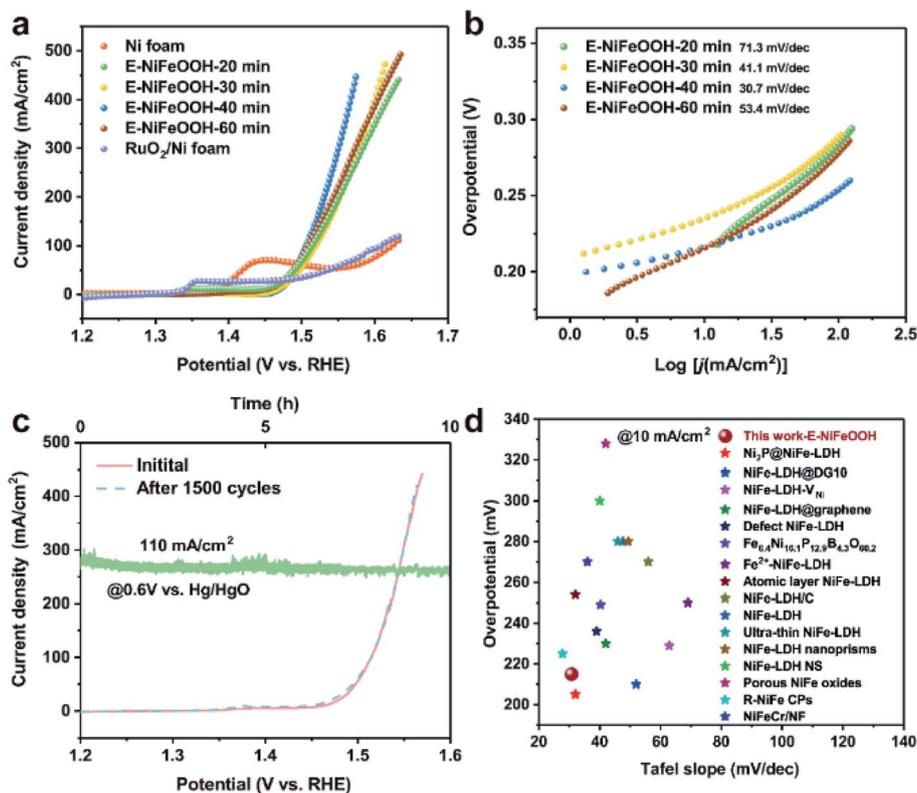
Fig. 4 (a and b) Polarization curves and corresponding Tafel plots of the Ni foam, E-NiFeOOH-20, 30, 40, 60 min and RuO<sub>2</sub>/NF electrodes for the OER. (c) Long-term stability tests and stability measurements of E-NiFeOOH-40 min. (d) Comparison of recent representative studies of NiFe-based OER electrocatalysts with their corresponding overpotentials at 10 mA cm<sup>-2</sup> and Tafel slope values (Table S3†).
