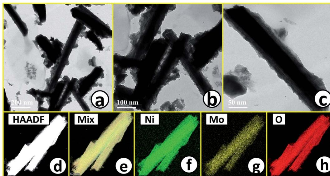
Fig. 4 (a)–(c) Low to high magnification HR-TEM images of  $\text{NiMoO}_4(\text{V}_\text{o})$ ; (d) is the HAADF image of rod-like  $\text{NiMoO}_4(\text{V}_\text{o})$  taken for the mapping analysis; (e)–(h) are the characteristic mapping results of mix, Ni K, Mo K, O K and respectively.
