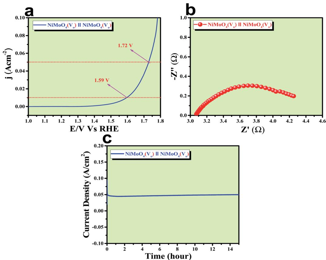
Fig. 10 (a) LSV curve of rod like  $\text{NiMoO}_4(\text{V}_o)$  as an anode and cathode in a two electrode system at a scan rate of  $2 \text{ mV s}^{-1}$ , (b) impedance spectra obtained at 400 mV overpotential, and (c) chronoamperometric outcomes for 15 hours.
