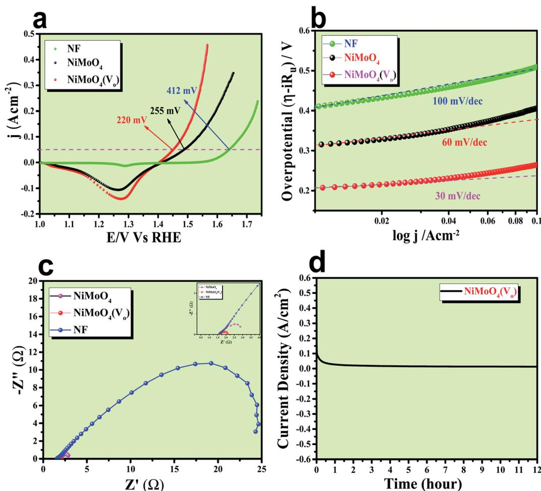
Fig. 7 (a) Is the backward CV of rod like  $\text{NiMoO}_4(\text{V}_\text{o})$  and  $\text{NiMoO}_4$  at a scan rate of  $5 \text{ mV s}^{-1}$ , (b) corresponding Tafel plot, (c) impedance spectra obtained at 300 mV overpotential and (d) chronoamperometric outcomes for 12 h.
