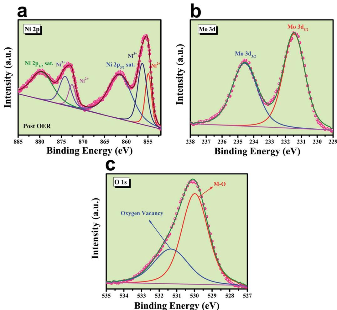
Fig. 12 Post XPS characterization of NiMoO<sub>4</sub>(V<sub>o</sub>): (a) high-resolution XPS spectra of Ni 2p orbitals, (b) XPS spectra of Mo 3d orbital and (c) deconvoluted XPS spectrum of O 1s orbitals.
