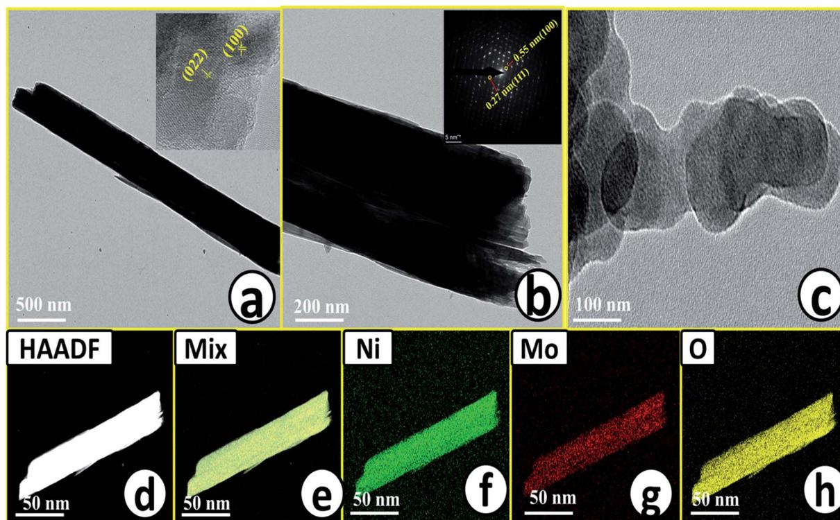
Fig. 3 (a) and (c) Low to high magnification HR-TEM images of  $\text{NiMoO}_4$ , inset of (a) and (b) are corresponding lattice fringes and SAED pattern respectively, (d) is the HAADF image of rod-like  $\text{NiMoO}_4$  taken for the mapping analysis, (e)–(h) are the characteristic colour mapping results of mix, Ni, Mo and O, respectively.
