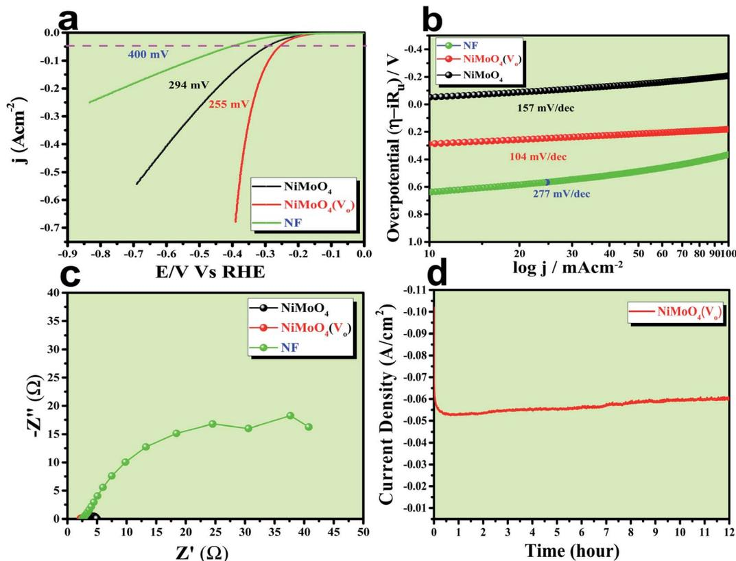
Fig. 9 (a) LSV curve of rod like  $\text{NiMoO}_4(\text{V}_o)$  and  $\text{NiMoO}_4$  at a scan rate of  $5 \text{ mV s}^{-1}$ , (b) corresponding Tafel plot, (c) impedance spectra obtained at 250 mV overpotential and (d) chronoamperometric outcomes for 12 hours.
