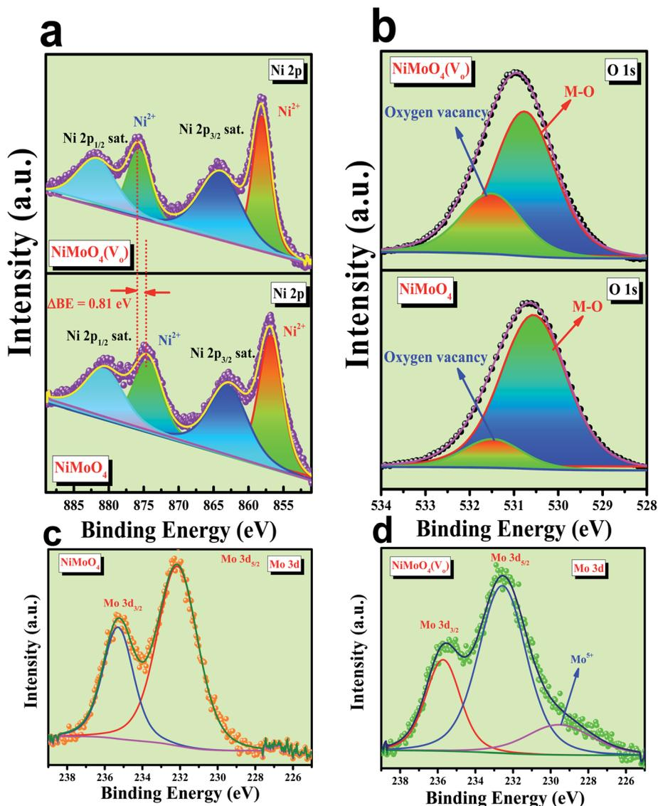
Fig. 5 (a) Combined high-resolution XPS spectra of Ni 2p orbitals for NiMoO<sub>4</sub> and NiMoO<sub>4</sub>(V<sub>o</sub>). (b) deconvoluted XPS spectrum of O 1s orbitals, (c) XPS spectra of Mo 3d orbital of NiMoO<sub>4</sub> and, (d) XPS spectra of Mo 3d orbital of NiMoO<sub>4</sub>(V<sub>o</sub>).
