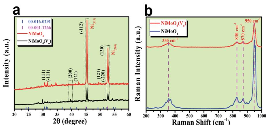
Fig. 1 (a) XRD patterns of rod shaped NiMoO<sub>4</sub> and NiMoO<sub>4</sub>(V<sub>o</sub>), (b) Raman spectra of rod shaped NiMoO<sub>4</sub> and NiMoO<sub>4</sub>(V<sub>o</sub>).
