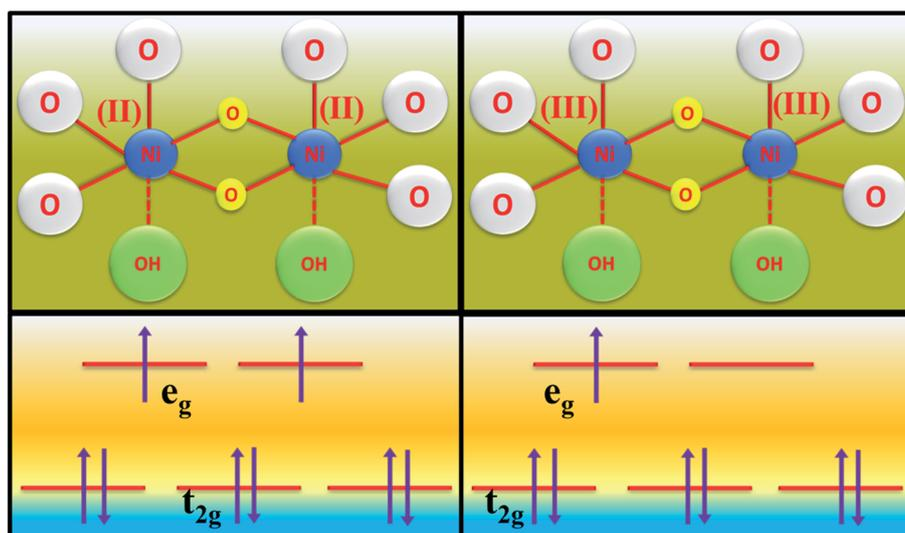
Scheme 2 Scheme of electron occupancy in different crystal field splitted orbitals of the Ni centre.
