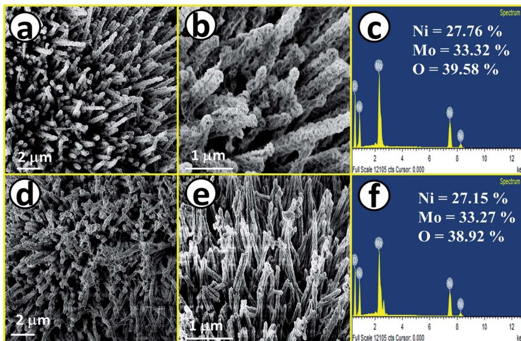
Fig. 2 (a) and (b) FE-SEM images of  $\text{NiMoO}_4$  nano-rods, (c) EDS spectrum of  $\text{NiMoO}_4$  in the FE-SEM mode, (d) and (e) FE-SEM images of  $\text{NiMoO}_4(\text{V}_o)$  nanorod and (f) EDS spectrum of  $\text{NiMoO}_4(\text{V}_o)$  in the FE-SEM mode.
