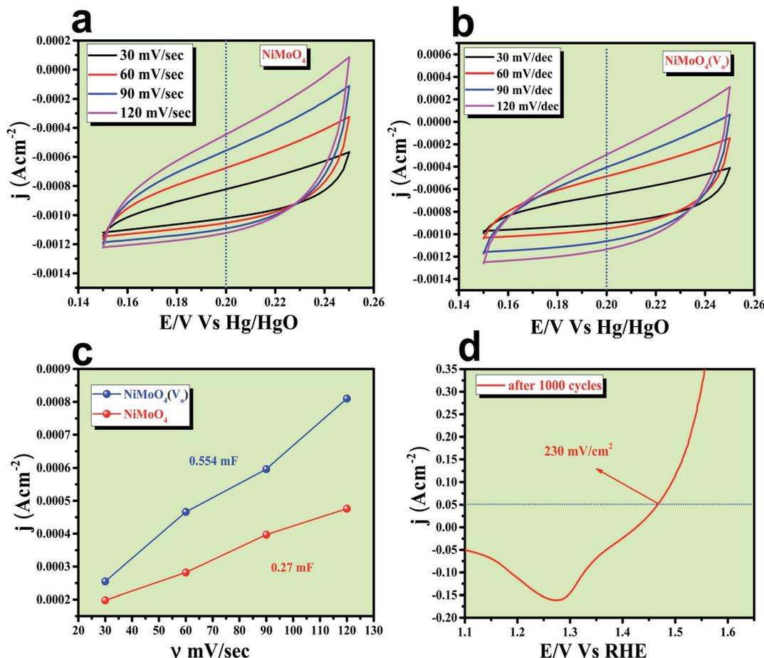
Fig. 8 (a) and (b) Are the CVs recorded for  $\text{NiMoO}_4$  and  $\text{NiMoO}_4(\text{V}_o)$  respectively in a non-faradaic region with increasing scan rate for the determination of ECSA from its double layer capacitance; (c) are the corresponding plots to the measure  $C_{dl}$ ; (d) backward CV after 1000 cycles of AD study.
