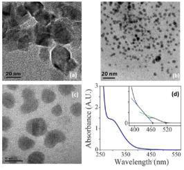
Fig. 8 TEM images of  $Ta_3N_5$  obtained by Ho et al.<sup>87</sup> (a) NPs obtained with  $TaCl_5$  and  $(TMS)_3N$  (scale 20 nm), (b) with  $Ta(NMe_2)_5$  and  $(TMS)_3N$  (scale 20 nm) (c) with  $TaCl_5$  and  $Li_3N$  (scale 10 nm). (d) Absorption spectrum of the obtained 10 nm  $Ta_3N_5$ . The inset showing the two limiting regimes. Adapted with permission from ref. 87. Copyright 2010 American Chemical Society.
