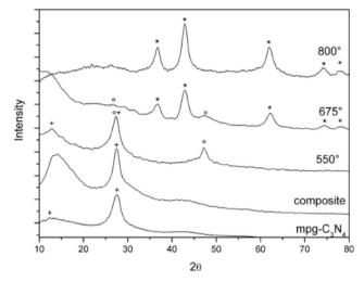
Fig. 6 Temperature-dependent powder XRD analysis of the  $TiO_2$  precursor/mpg- $C_3N_4$  composites. (+) represents mpg- $C_3N_4$ ; (o),  $TiO_2$ ; and (\*), TiN. Reprinted from ref. 66 with permission from John Wiley and Sons, Copyright 2007.
