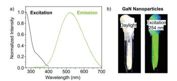
Fig. 20 (a) Emission spectrum at 274 nm and excitation spectrum at 523 nm of the synthesized GaN. (b) Photographs of the as synthesized GaN NCs in daylight and under excitation at 254 nm. Reprinted from ref. 168 with permission from the Royal Society of Chemistry.
