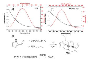
Fig. 18 UV-Vis absorption and photoluminescence spectra of Cu<sub>7</sub>N obtained via (a) PPC and (b) Cu(NO<sub>3</sub>)<sub>2</sub>·3H<sub>2</sub>O method. Reprinted from ref. 124 with permission from the Royal Society of Chemistry. (c) Reaction mechanism proposed for Cu<sub>3</sub>N formation from the reaction of pyrrole-2carbaldpropyliminato Cu(II) (PPC) and ODA shown below. 124
