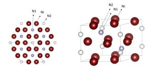
Fig. 9 Crystal structure of Ni $_3$ N. The nickel atoms are represented in dark red and the nitrogen atoms in cyan and white. Structures plotted using VESTA.  $^{48}$  Cif file obtained from ref. 89.
