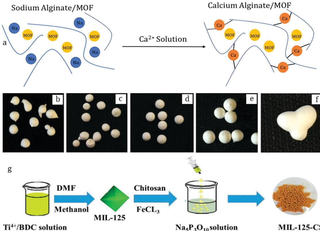
Fig. 17 Schematic representation of the "molecular gastronomy" method (a). UiO-66 beads (b–f) prepared by Lee *et al.*<sup>146</sup> showing the effect of the concentration of the gelation solution on the final shape of the beads: b – 0.2% (w/v); c – 0.5% (w/v); d – 2.0% (w/v); and e and f – 10% (w/v). Copyright 2020 Elsevier. Preparation of MIL-125(Ti) beads (g) with chitosan as a binding biopolymer.<sup>149</sup> Copyright 2018 MDPI.
