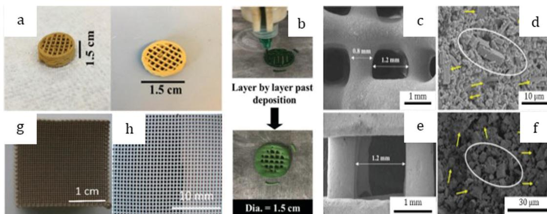
Fig. 11 Photographs of objects 3D-printed *via* the DIW method: monoliths (a) prepared by Thakkar *et al.*<sup>107</sup> Copyright 2017 American Chemical Society. Ni(bdc)(ted)<sub>0.5</sub> monolith (b) with its SEM images (c and d) and SEM images of ZIF-7 (e and f) monoliths prepared by Thakkar *et al.*<sup>108</sup> Copyright 2018 American Chemical Society. ZIF-8 monolith (g) and its optical image (h) made by Lefevre *et al.*<sup>112</sup> Copyright 2019 American Chemical Society.
