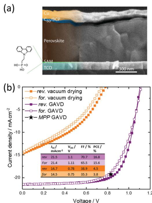
**Fig. 4** (a) Solar cell architecture on p–i–n architecture. The Perovskite layer is inkjet-printed with the GAVD process. (b) Current density–voltage characteristics and of inkjet-printed perovskite solar cells on SAM using vacuum drying and GAVD method. Value for mpp-tracking (16%) is the average over 300 s of tracking the power output.
