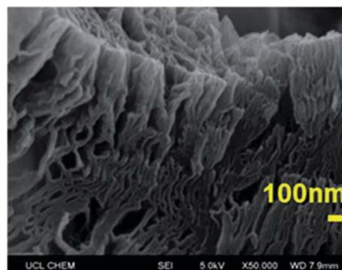
Fig. 5 SEM micrograph of exfGO-D<sub>7.0</sub>TETA, exfoliated graphene-oxide impregnated with 7.0 g g<sup>-1</sup> TETA. Reproduced from ref. 94 with permission from the Royal Society of Chemistry.
