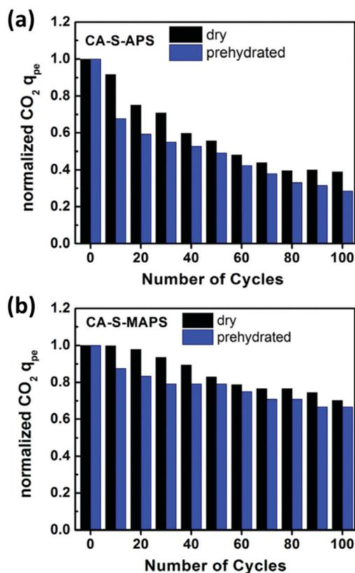
Fig. 24 Comparison of the cyclic CO<sub>2</sub> capacity of dry fibres and pre-hydrated fibres in 200 ppm SO<sub>2</sub> in 10% CO<sub>2</sub>/N<sub>2</sub> at 35 °C of; (a) primary amine-grafted and; (b) secondary amine-grafted fibres. CO<sub>2</sub> capacities normalised to adsorbents' initial CO<sub>2</sub> capacity  $q_{pe,0}$  before exposure degradation. Reprinted from ref. 36 Copyright (2015), with permission from Elsevier.
