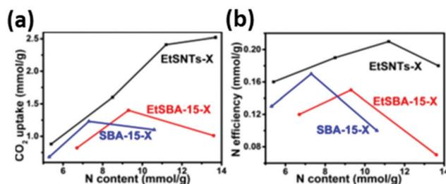
Fig. 10 The relationship between (a) CO<sub>2</sub> uptake and (b) N efficiency with N content of PEI/silica composites at 30 °C and 0.1 bar CO<sub>2</sub>. Adapted with permission from ref. 125. Copyright 2020, John Wiley and Sons.
