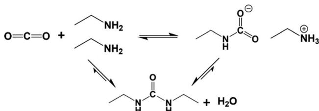
Fig. 21 Relationship between formation of carbamate and urea species during CO<sub>2</sub> adsorption-desorption under dry conditions. Adapted with permission from ref. 123. Copyright (2010) American Chemical Society.
