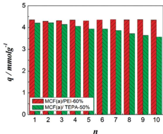
Fig. 17 CO<sub>2</sub> adsorption capacity of cyclic CO<sub>2</sub> adsorption–desorption of MCF(a)/PEI-60% and MCF(a)/TEPA-50%. Reprinted with permission from ref. 141. Copyright (2012) American Chemical Society.
