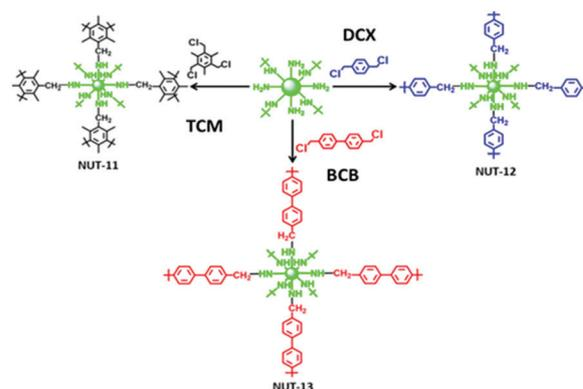
Fig. 7 Cross-linking of PEI with 2,4,6-tris(chloromethyl)mesitylene (TCM), 4,4'-bis-(chloromethyl)-1,1'-biphenyl (BCB), and *p*-dichloroxylylene (DCX). Reprinted with permission from ref. 115. Copyright (2018) American Chemical Society.
