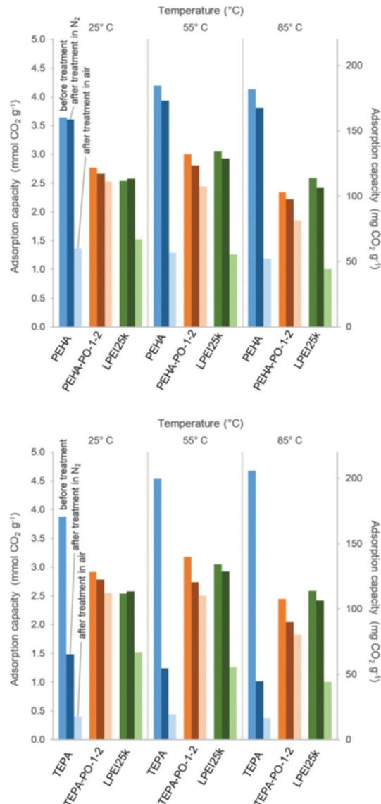
**Fig. 20** Effect of propylene oxide modification of TEPA- and PEHA-based adsorbents on CO<sub>2</sub> adsorption under 95% CO<sub>2</sub> in 25, 55, and 85 °C for 3 h before and after treatment under air or N<sub>2</sub> at 100 °C for 20 h. Comparison with LPEI25k/50S. Reproduced with permission from ref. 70. Copyright 2019, John Wiley and Sons.
