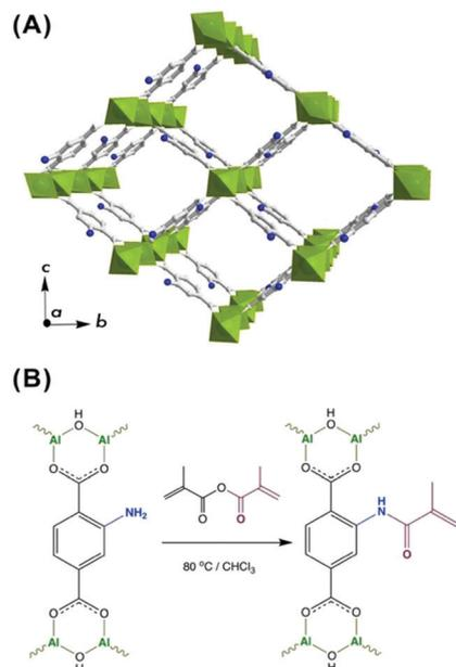
**Fig. 1** (A) Representation of MIL-53(Al)-NH<sub>2</sub> structure in the open pore configuration, where AlO<sub>6</sub> polyhedra are depicted in green, and grey and navy are carbon and nitrogen atoms, respectively. (B) Scheme of post-synthetic modification of MIL-53(Al)-NH<sub>2</sub> structure with methyl methacrylate anhydride.
