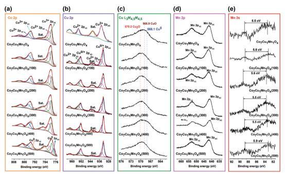
Fig. 3 XPS spectra of the unreduced  $Co_7Cu_1Mn_1O_x$  catalyst and the  $Co_7Cu_1Mn_1O_x(100, 200, 300, and 500)$  catalysts. (a) Co 2p XPS, (b) Cu 2p XPS, (c) Cu  $L_3M_{4.5}M_{4.5}$  AES spectra, (d) Mn 2p XPS, and (e) Mn 3s XPS, respectively.
