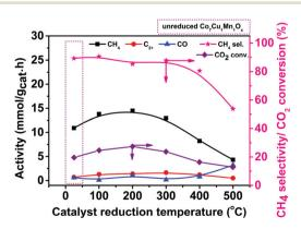
**Fig. 4** Effect of the reduction temperature of the  $Co_7Cu_1Mn_1O_x(T)$  catalysts on the catalytic performances of photothermal  $CO_2$  reduction. Reaction conditions: catalyst 50 mg,  $CO_2/H_2/N_2$  10%/30%/60%, 200 °C, 3 h, and 300 W Xe lamp full irradiation.
