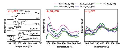
Fig. 6 H<sub>2</sub>-TPR(a), CO<sub>2</sub>-TPD (b), and H<sub>2</sub>-TPD (c) tests for the different catalysts.
