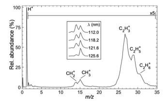
Fig. 3 Time-of-flight mass spectrum of ions formed following photoexcitation of a jet-cooled sample of  $C_2H_6$  seeded in He at  $\lambda=121.6$  nm ( $h\nu=10.19$  eV). Inset: expanded spectra illustrating the  $\lambda$ -dependence of the m/z 14 ( $CH_2^+$ ) and m/z 15 ( $CH_3^+$ ) peak intensities.
