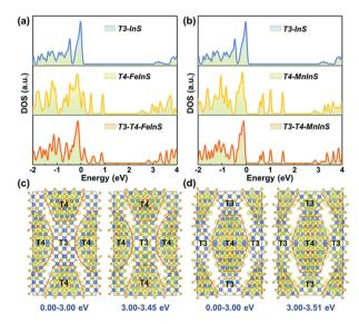
Fig. 3 (a) DOS of T3-InS, T4-FeInS, and T3-T4-FeInS. (b) DOS of T3-InS, T4-MnInS, and T3-T4-MnInS. Band-decomposed charge densities in energy ranges of 0.00-3.00 eV and 3.00-3.45 eV for (c) T3-T4-FeInS and (d) T3-T4-MnInS. The isosurface value is 0.001 eV Å $^{-3}$ . S, In, Fe, and Mn atoms are presented with yellow, brown, blue, and violet circles, respectively.
