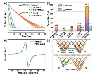
Fig. 6 (a) PL decay curves of *T3-T4-MnInS*, *T4-MnInS*, and the mechanical mixture of *T3-InS* and *T4-MnInS* obtained for pulsed 372 nm (or 469 nm) excitation and 631 nm emission at RT. (b) Average PL decay lifetimes of *T3-T4-MnInS* and other T4-MnInS-cluster-based chalcogenides reported previously. (c) EPR spectra of *T4-MnInS* and *T3-T4-MnInS*. (d) Schematic structural difference between T4-T4 and T4-T3.
