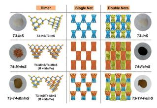
Fig. 2 Images of T3-InS, T4-FeInS, T4-MnInS, T3-T4-FeInS and T3-T4-MnInS, as well as the corresponding structures.
