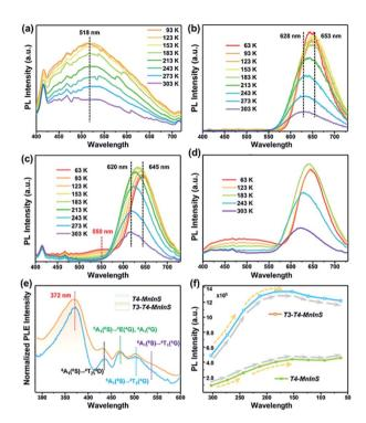
Fig. 5 PL spectra of (a) T3-InS, (b) T4-MnInS, (c) T3-T4-MnInS and (d) a mechanical mixture of T3-InS and T4-MnInS (1 : 1, mol mol $^{-1}$ ) upon excitation at 375 nm and different temperatures. (e) Normalized PLE spectra of T4-MnInS and T3-T4-MnInS for emission at 631 nm at room temperature. (f) Temperature-dependent PL intensity of T4-MnInS and T3-T4-MnInS.
