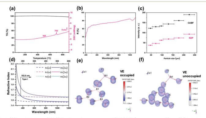
Fig. 2 (a) Thermal behaviour of CABF. (b) The diffuse reflectance spectrum of CABF. (c) PSHG measurements at 1064 nm. (d) Calculated type I phase-matching condition of CABF. Dashed lines: refractive-indices of fundamental light. Solid lines: refractive-indices of second-harmonic light. The  $\lambda_{SH}$  of CABF is estimated by satisfying  $n_{Z(\omega)} = n_{X(2\omega)}$ . The SHG-weighted electron density maps of the occupied (e) and unoccupied (f) states in the VE process.
