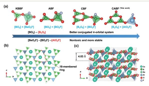
Fig. 1 (a) The structural evolution from  $KBe_2BO_3F_2$  to  $CsAlB_3O_6F$ . (b) The 2D  $[AlB_3O_6F]_{\infty}$  layer of CABF. (c) Crystal structure of CABF.
