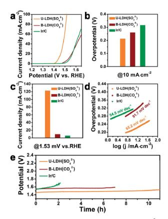
Fig. 3 (a) Linear sweep voltammetry OER curves of U-LDH( ${\rm SO_4}^{2-}$ ), B-LDH( ${\rm CO_3}^{2-}$ ) and commercial Ir/C. (b) Overpotentials of different catalysts at the current density of 10 mA cm $^{-2}$ . (c) Current densities of different catalysts at 1.53 V *versus* RHE. (d) Tafel plots of different catalysts. (e) Chronopotentiometry tests of U-LDH( ${\rm SO_4}^{2-}$ ), B-LDH( ${\rm CO_3}^{2-}$ ) and commercial Ir/C in 1 M KOH at 10 mA cm $^{-2}$ .
