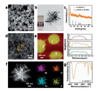
Fig. 1 (a) SEM image, (b) TEM image, (c) PXRD patterns, (d) HRTEM image, (e) AFM image and height profiles, (f) HAADF-STEM image and EDX elemental mappings, (g) FT-IR spectrum of the U-LDH(SO<sub>4</sub><sup>2-</sup>). The inset in (b) shows the Tyndall light scattering of the U-LDH(SO $_4^2$ in aqueous solution.
