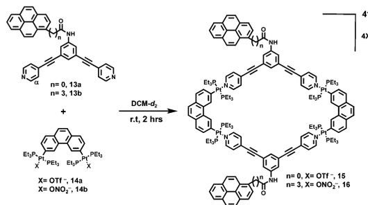
Scheme 4 Synthesis of pyrene-functionalized molecular rhomboids **15** and **16**.
