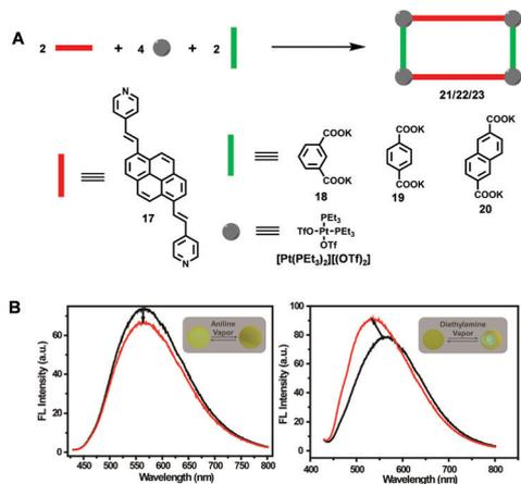
**Fig. 1** The construction of pyrene-based metallocycles **21–23** via coordination-driven self-assembly (A) and the sensing performance of **22**-based fluorescent films towards aniline (left) and diethylamine (right) (B). Adapted with permission from ref. 10. (Copyright 2019 American Chemical Society.)
