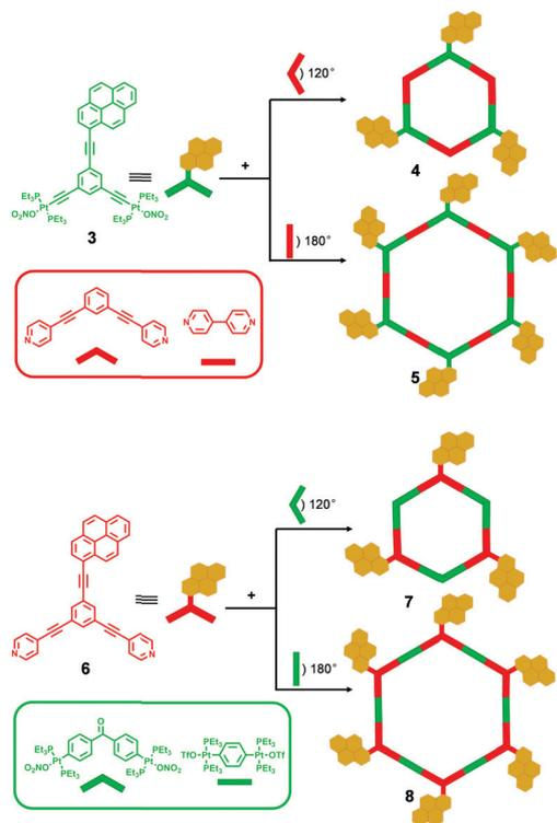
Scheme 2 Coordination-driven self-assembly of multipyrene hexagonal metalocycles **4**, **5**, **7**, and **8**.
