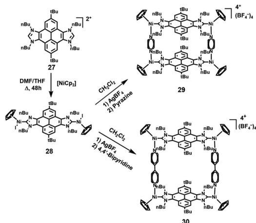
Scheme 5 The synthesis of nickel-cornered metallo-rectangles **29** and **30**.
