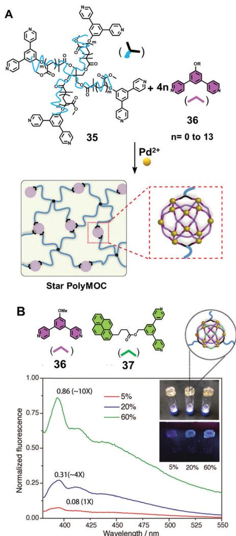
**Fig. 6** The preparation of the star PolyMOCs via a three-component assembly approach (A) and the incorporation of pyrene moieties as functional groups (B). Adapted with permission from ref. 20. (Copyright 2017 Wiley-VCH.)
