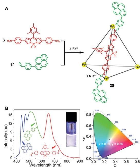
**Fig. 7** The construction of the tetrahedral metallogel **38** via the subcomponent self-assembly approach (A) and the white light emission of the complex of the resultant metallogel and perylene (B).
