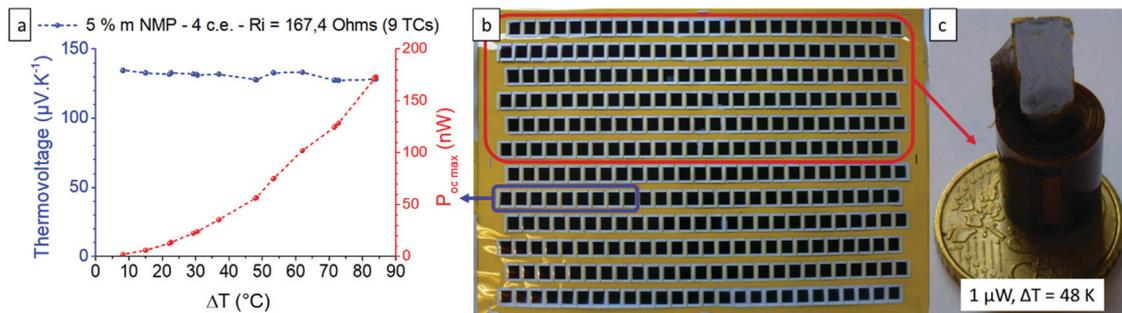
Fig. 5 (a) Thermovoltage and power density measured for a 9-thermocouples TEG module (b) picture of 312 spray-coated legs on a 25  $\mu\text{m}$  thick polyimide foil (c) 3D TEG composed of 156 linked and rolled thermocouples ( $R_i = 2.9 \text{ k}\Omega$ ).
